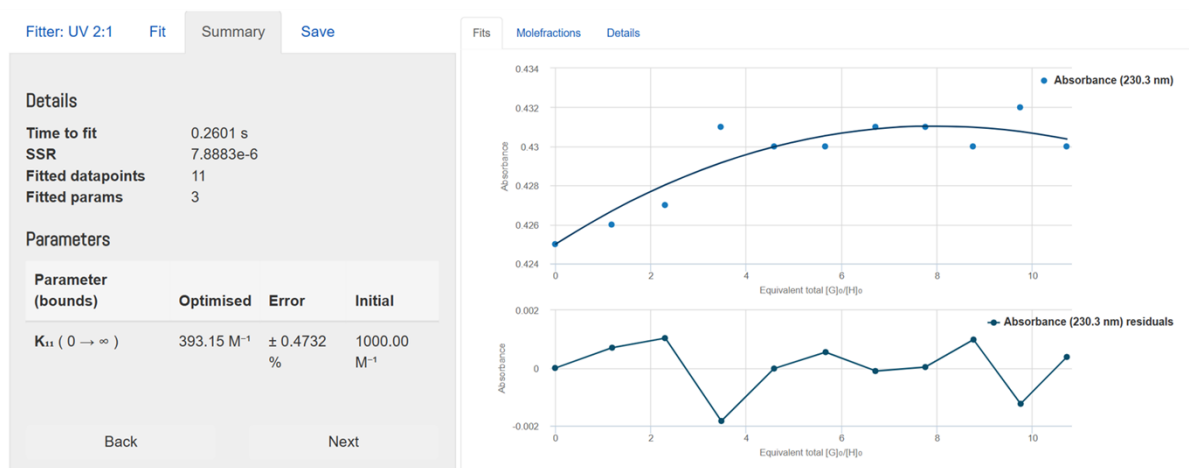
Figure S45: UV-vis absorbance titration data (at 230.3 nm) of receptor 2c ( 10^{-5} M) observed upon the addition of TBAClO 4 ( 10^{-3} in CH 3 CN) and fitted to 2:1 (H:G) binding model of BindFit v0.5.
