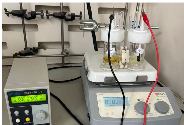
Figure S4. Electrochemical reaction in divided cell. Reaction conditions: benzyl alcohol (1.5 ml), TFA (10 mol %), n Bu 4 NBF 4 (0.1 M), CH 3 CN (6.5 mL) in anodic compartment, o -nitrophenol (1.0 mmol), TFA (10 mol %), n Bu 4 NBF 4 (0.1 M), and CH 3 CN (8 mL) cathodic compartment, H-cell with Nafion N117 membrane, constant current 20 mA, room temperature, 8 h.
