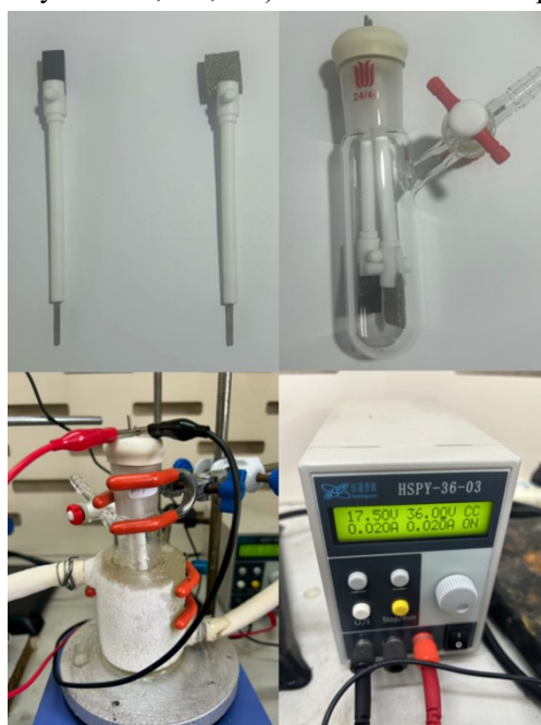
Figure S1. Photographic Guide for Electrochemical Reaction. Glassy carbon plate (anode, 10 \times 20 \times 3 mm), nickel foam plate (cathode, 15 \times 20 \times 3 mm), undivided electrochemical cell.
