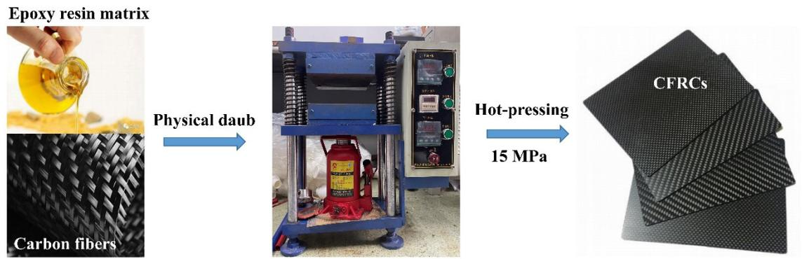
**Fig. S4.** The process of forming prototypical CFRCs was used in this work (50.0 wt.%).
