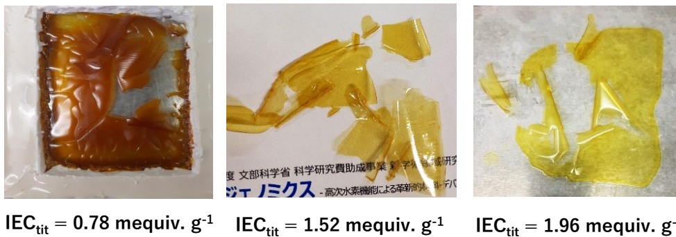
Fig. S8 Photos of cracked QmTPh-Pip membranes.
