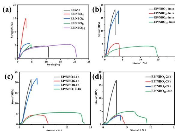
**Fig. 3** (a) Tensile test of EP/651 and EP/ $\text{NBO}_n$  at room temperature, (b) Tensile test of EP/ $\text{NBO}_n$  after soaking in liquid nitrogen for 1 min, (c) Tensile test of EP/ $\text{NBO}_n$  after soaking in liquid nitrogen for 1 h, (d) Tensile test of EP/ $\text{NBO}_n$  after soaking in liquid nitrogen for 24 h.
