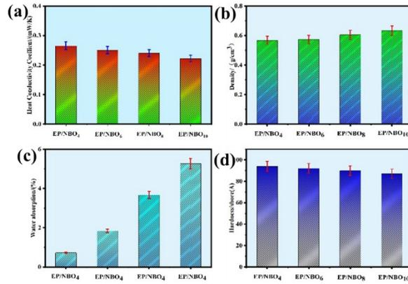
**Fig. 4** (a)Thermal conductivity of EP/NBO<sub>n</sub>,(b)Density of EP/NBO<sub>n</sub>,(c)Water absorption of EP/NBO<sub>n</sub>,(d)Hardness of EP/NBO<sub>n</sub>.
