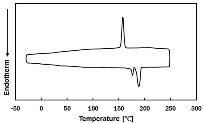
Figure. S5. DSC curve of 1,4-DMSB-MVSB.
