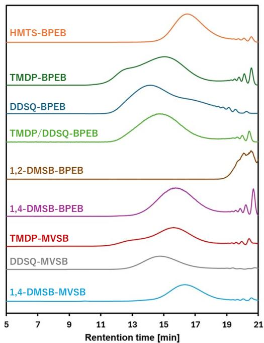
Figure. S4. SEC curves of the silicon-containing hydrocarbon-based polymers.
