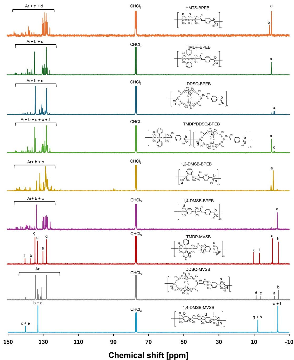
Figure. S2.  $^{13}\text{C}$  NMR spectra of the silicon-containing hydrocarbon-based polymers.
