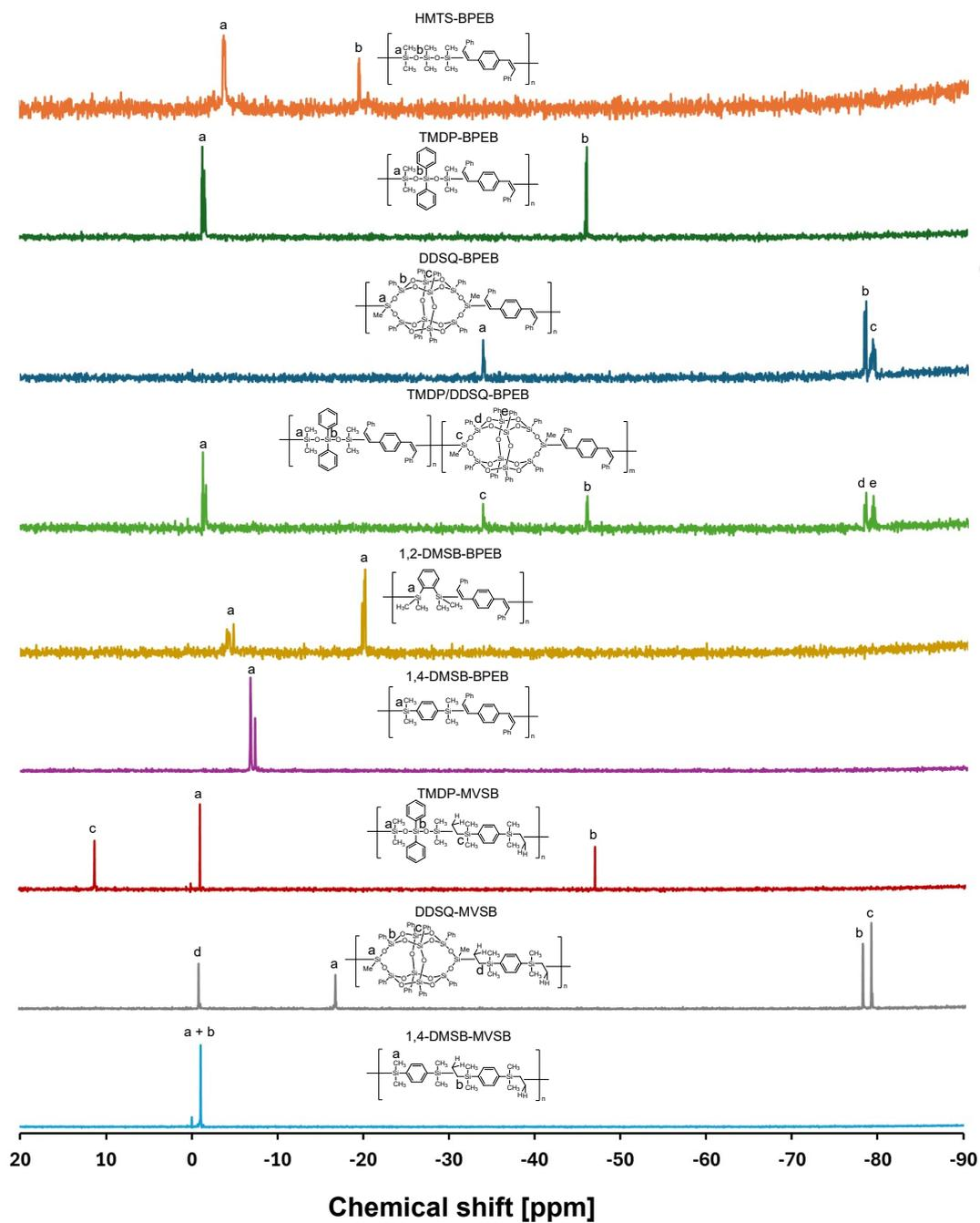
Figure. S3.  $^{29}\text{Si}$  NMR spectra of the silicon-containing hydrocarbon-based polymers.
