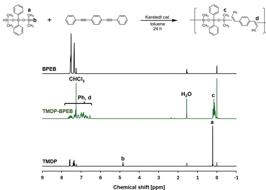
Figure. S1. <sup>1</sup>H NMR spectra of TMDP-BPEB.
