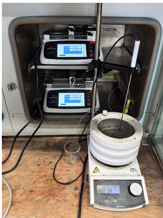
Figure S1. The continuous flow set-up for irreversible polyaddition.
