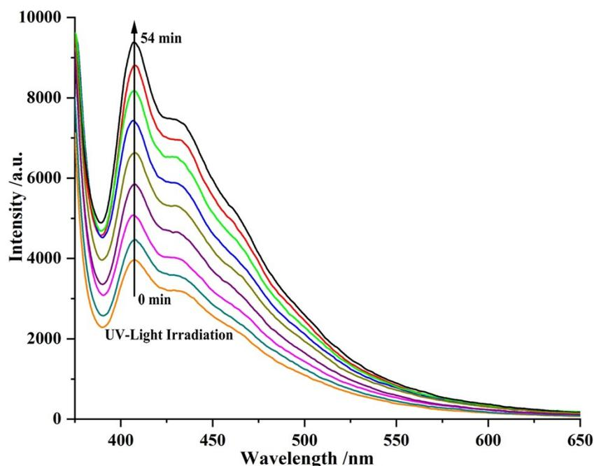
**Figure S17.** Fluorescence spectrum ( $\lambda_{\text{ex}} = 390$  nm) of ionic azo-homopolymer, **IAzoC<sub>0</sub>HP** dissolved in THF solution with the concentration of 0.005 M before and after UV-light irradiation, corresponding to the irradiation time in Figure 3.
