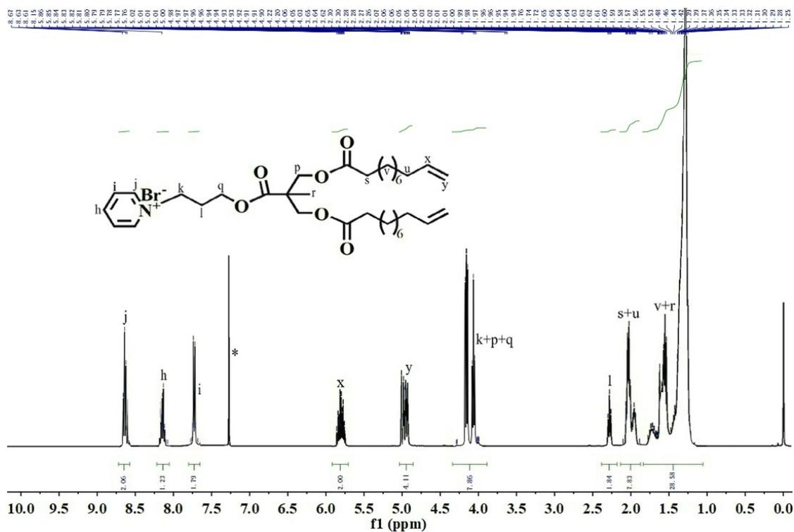
Figure S20. <sup>1</sup>H NMR spectrum of ionic diene monomer, Py-BrM.
