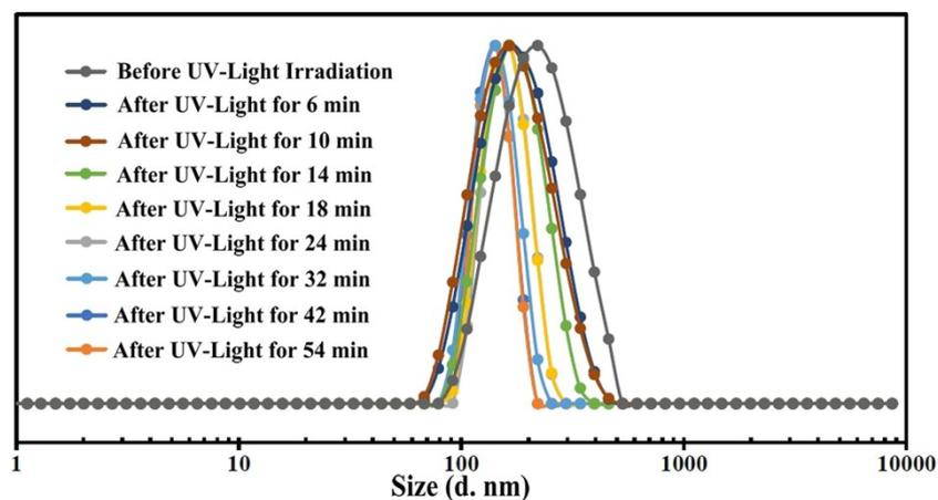
**Figure S16.** DLS curves of the morphology evolution of toroids from **IAzoC<sub>0</sub>HP** after UV-light irradiation with different time, corresponding to TEM images in Figure 3.
