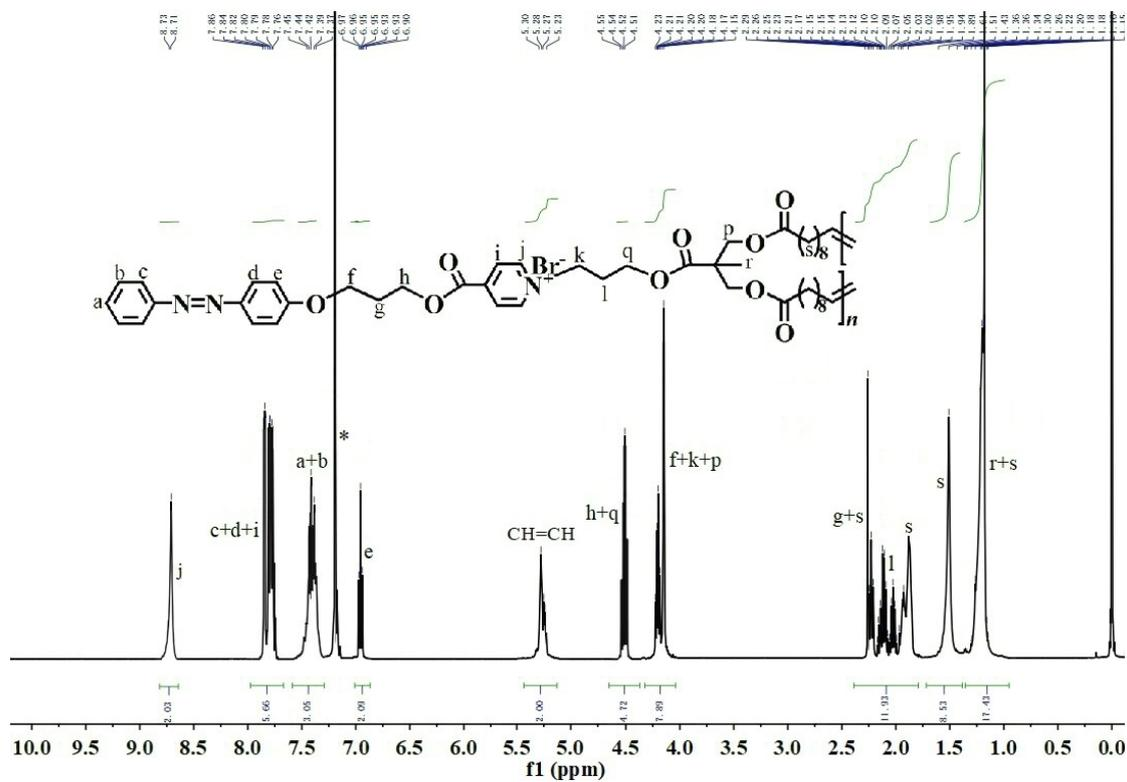
Figure S10. <sup>1</sup>H NMR spectrum of ionic azo-homopolymer, IAzoC<sub>3</sub>HP.
