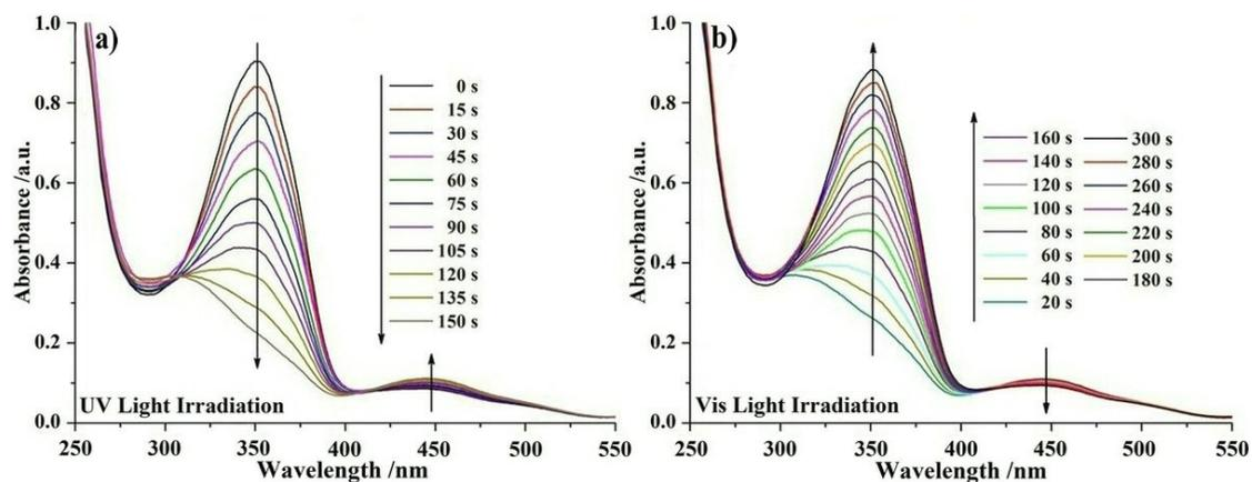
**Figure S22.** UV–Vis spectra of azo-homopolymer, **AzoHP** in diluted THF solutions with the concentration of  $2.5 \times 10^{-5}$  mol/L. Absorbance changes with (a) UV-light and (b) Vis-light irradiation times.
