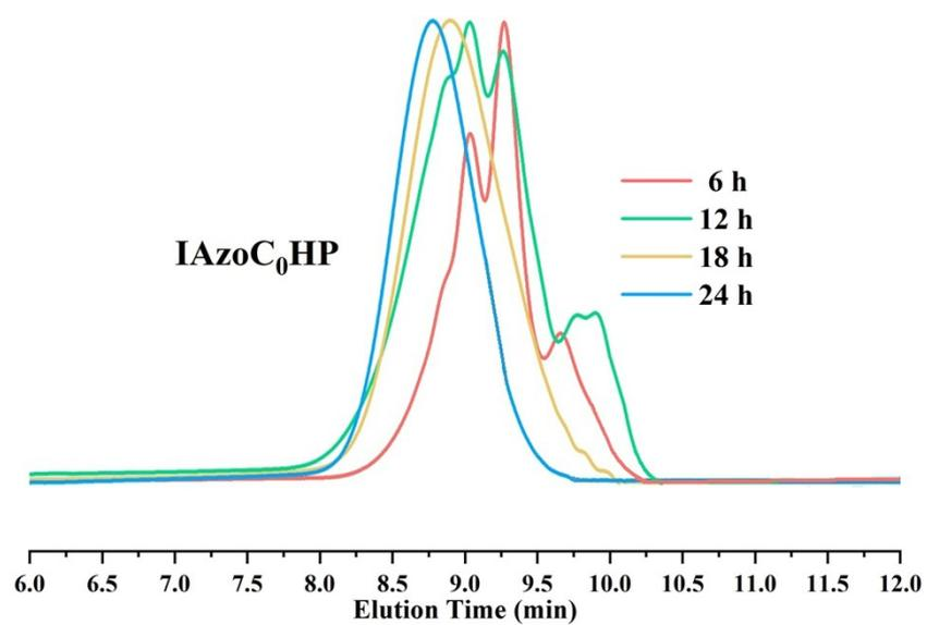
**Figure S12.** GPC traces of ionic azo-homopolymer, IAzoC<sub>0</sub>HP with different ADMET polymerization times.
