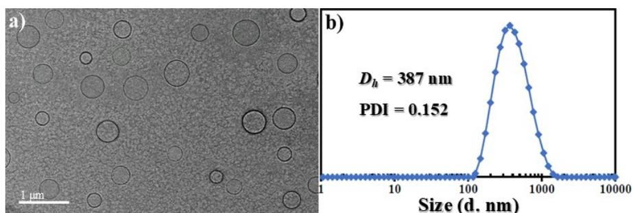
**Figure S15.** (a) TEM image and (b) corresponding DLS result of polymeric toroid self-assembled from **IAzoC<sub>0</sub>HP** solution stored for two weeks with the initial concentration of 0.03 M.
