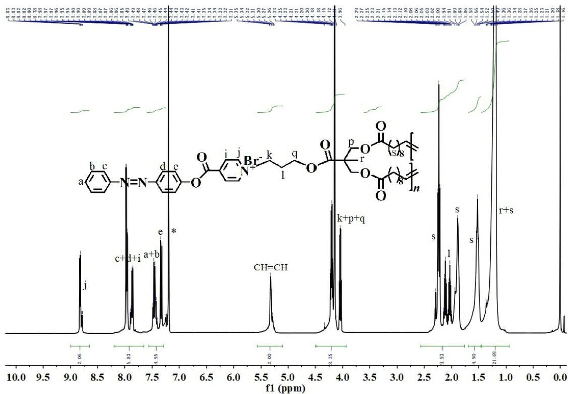
Figure S9. <sup>1</sup>H NMR spectrum of ionic azo-homopolymer, IAzoC<sub>0</sub>HP.
