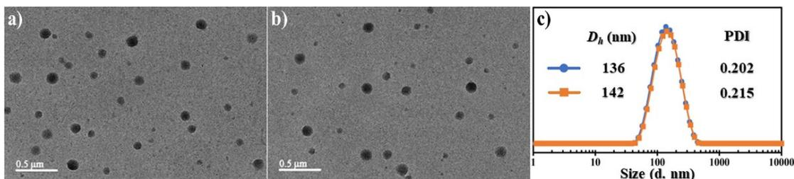
**Figure S23.** The self-assembly of pyridinium bromide-homopolymer, **Py-BrHP** to form micelles at initial concentration of 0.005 M. (a, b) TEM images of micelles before and after UV-light irradiation. (c) DLS analysis of the corresponding micelles in (a, b).
