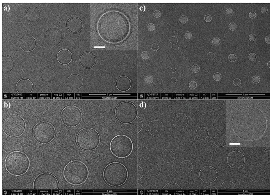
**Figure S14.** SEM images displaying self-assembled nanostructures of IAzoC<sub>p</sub>HPs
