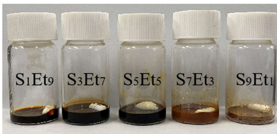
Figure S5. Digital photographs of reaction mixtures with varying weight ratios of sulfur to 2-ethyl-2-oxazoline after heating at 160 °C for 10 minutes and cooling.
