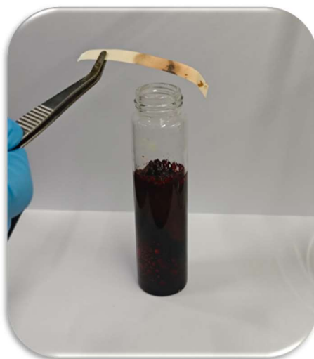
Figure S16. Lead acetate test detection of H 2 S generation in EUO-sulfur reaction at 160 °C.
