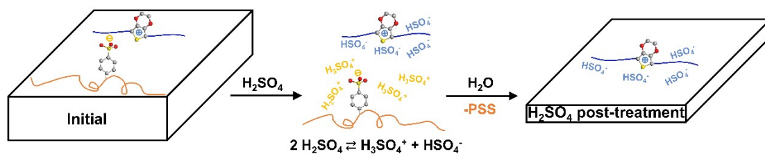
Fig. S17 Schematic illustration of the \text{H}_2\text{SO}_4 post-treatment mechanism.
