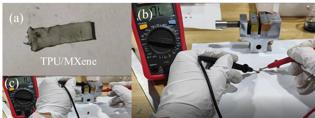
Figure S15. (a) Physical picture of TPU/MXene composite film. (b) The composite film is non-conductive, and the multimeter shows 0. (c) Test conductive metals with a multimeter
