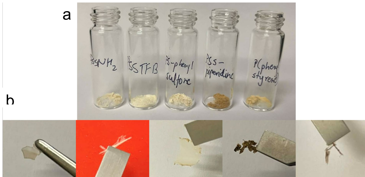
Figure S15. Processability of functionalized polymers. (a) Powder form of functionalized polymers (b) Hot-pressed functionalized polymers. From left to right: polystyrene sulfonamide, polystyrene trifluorobutyl sulfone, polystyrene phenyl sulfone, polystyrene sulfonyl piperidine, polyphenyl styrene.
