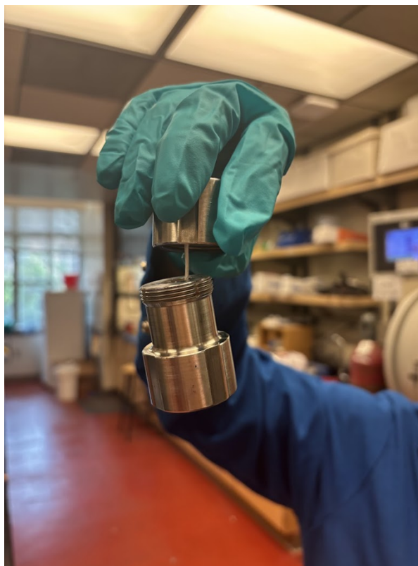
Figure S29: Image of UHMW AB poly( t BA- b -EA) ( Table 3 , entry 6) taken upon opening the milling jar. Approximately 2 g of polymer was capable of supporting the lower part of the 5 mL jar (mass = 253 g).
