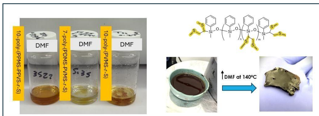
Figure S29- Solubility of synthesised polymers in DMF showing complete dissolution of 10-poly(PPMS-PPVS-r-S) and partial solubility of 5-poly(PDMS-PVMS-r-S) and of 10-poly(PVMS-r-S) (left). Removal of DMF from the dissolved 10poly(PPMS-PPVS-r-S) followed by heating at 140°C regenerates a cohesive solid network (right).
