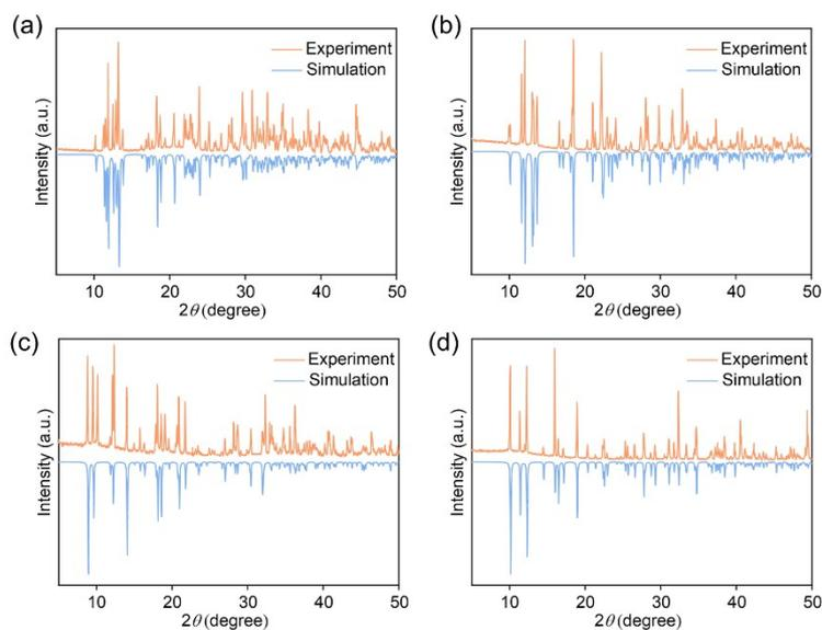
**Fig. S1.** PXRD patterns of compound R3PBKC (a), 3PBKC (b), PBC (c) and 3MPBKC (d) at 298 K.
