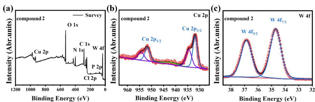
**Figure S9.** (a) XPS survey, (b) Cu 2p and (c) W 4f high-resolution XPS spectra of compound **2**.
