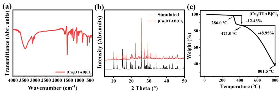
**Figure S15.** (a) IR spectrum of  $[\text{Cu}_3\text{DTAB}]\text{Cl}_3$ ; (b) XRD patterns of  $[\text{Cu}_3\text{DTAB}]\text{Cl}_3$ ; (c) TG curve of  $[\text{Cu}_3\text{DTAB}]\text{Cl}_3$ .
