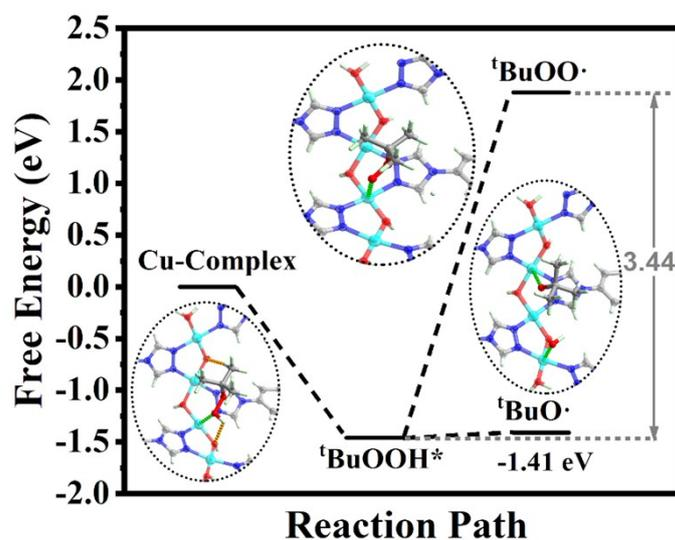
**Figure S20.** The adsorption energies of the *t*-BuOO• and *t*-BuO• species over Cu-DTAB complex.
