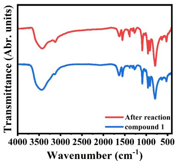
**Figure S21.** IR spectra of compound **1** before and after catalytic reaction.
