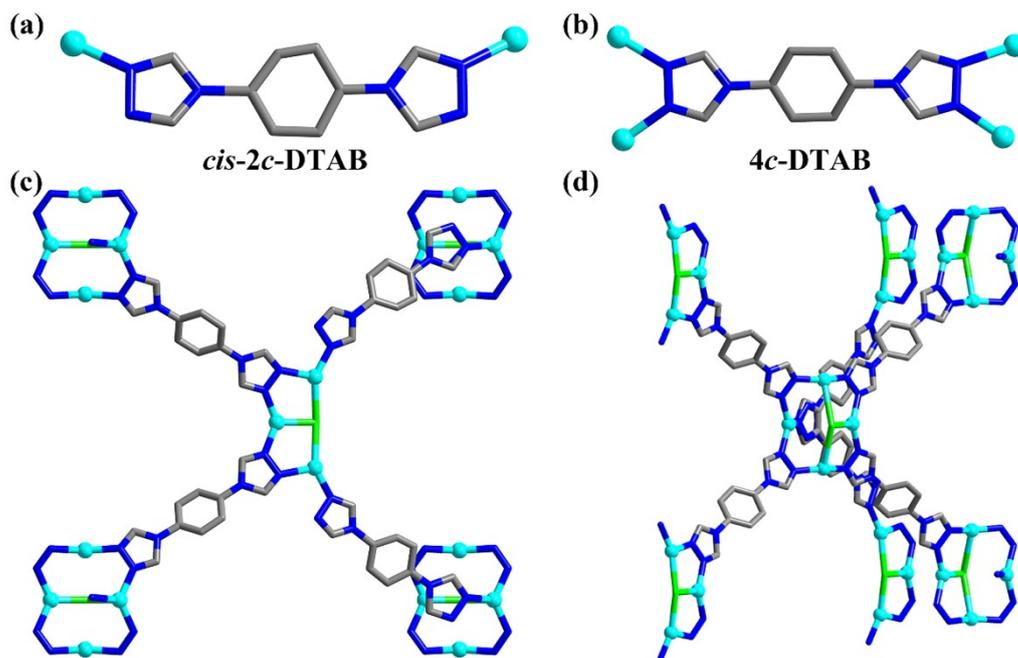
**Figure S7.** (a) Coordination mode of *cis*-2*c*-DTAB in compound **2**; (b) Coordination mode of 4*c*-DTAB in compound **2**; (c) Coordination mode of {Cu<sub>3</sub>Cl} unit; (d) Coordination mode of {Cu<sub>4</sub>Cl} unit in compound **2**.
