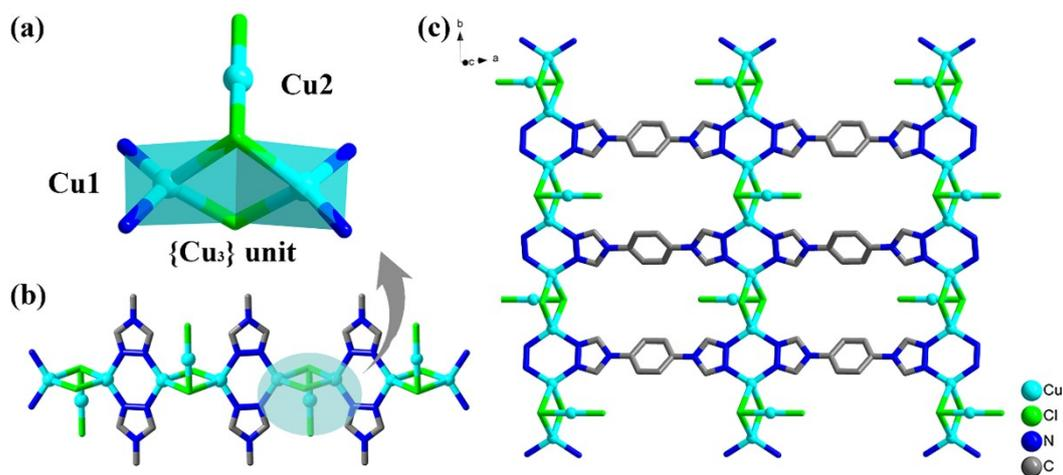
**Figure S14.** (a)  $[\text{Cu}_3^{I_3}(\mu_2\text{-Cl})_2\text{Cl}(\text{N-N})]$  unit in  $[\text{Cu}_3\text{DTAB}]\text{Cl}_3$ ; (b) 1-D metal-organic chain in  $[\text{Cu}_3\text{DTAB}]\text{Cl}_3$ ; (c) 2-D metal-organic network of  $[\text{Cu}_3\text{DTAB}]\text{Cl}_3$ .
