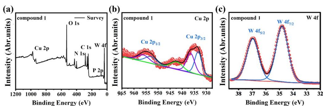
**Figure S2.** (a) XPS survey, (b) Cu 2p and (c) W 4f high-resolution XPS spectra of compound **1**.
