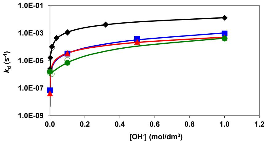
**Figure S13.** Pseudo-first order rate constants ( $k_d$ ) characterizing the transchelation reaction of **[Fe(NOTA)]**, **[Fe(DETA)]**, **[Fe(UNTA)]** and **[Fe(DOTRA)]** complexes with HBED ligand ( $[FeL]=0.2\text{ mM}$ ,  $[HBED]=2.0$  ( $\oplus$ ,  $\bullet$ ,  $\square$ ,  $\bowtie$ ) and  $4.0\text{ mM}$  ( $*$ ,  $\bowtie$ ),  $I=[Na^+]+[H^+]=0.15\text{ M}$ ,  $[H^+] \leq 0.15\text{ M}$ ,  $25^\circ C$ ).
