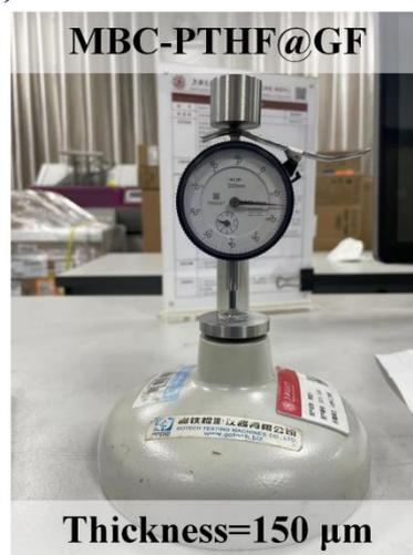
**Figure S6.** Thickness tests of MBC-PEG@GF CGPE and MBC-PTHF@GF CGPE.
