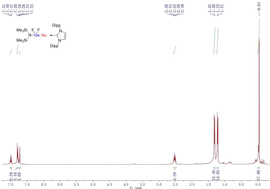
**Fig. S31**  $^1\text{H}$  NMR spectrum of **8** in  $\text{CDCl}_3$ .
