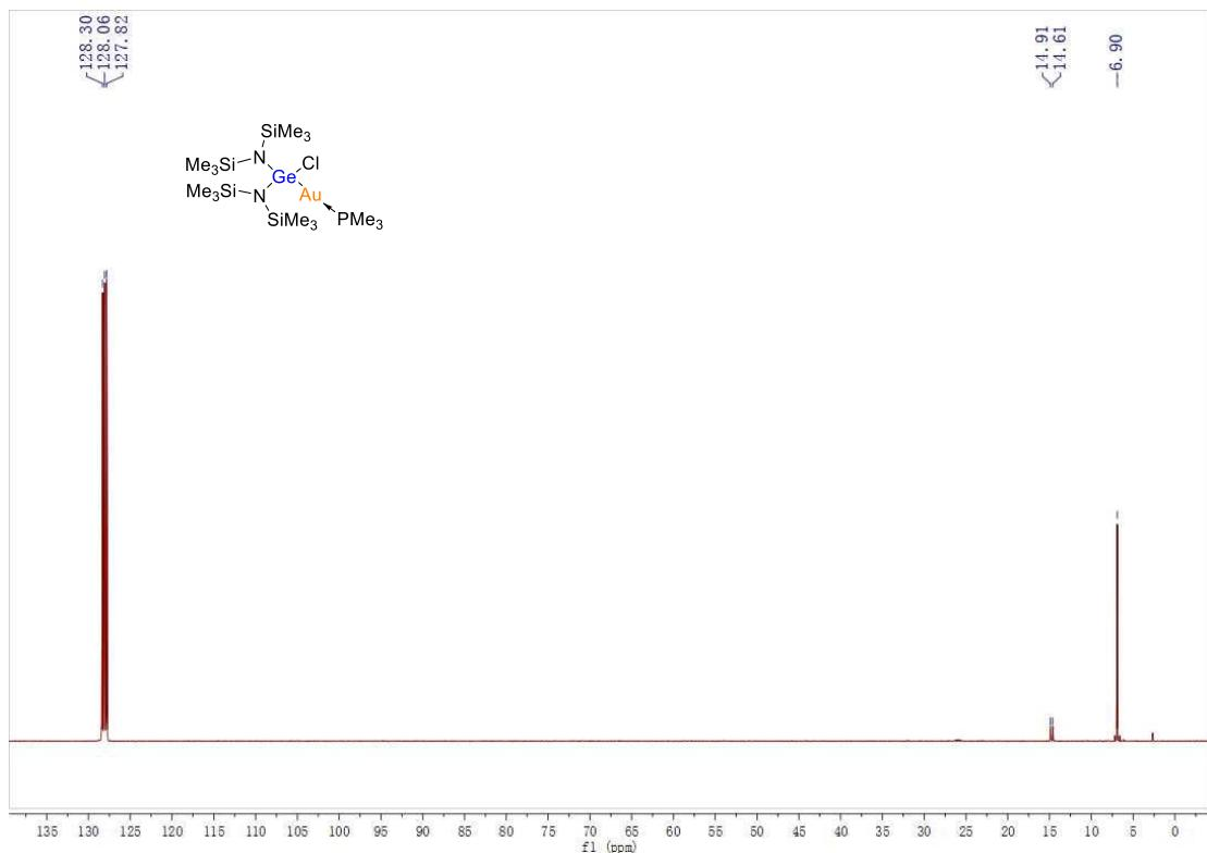
**Fig. S22**  $^{13}\text{C}$  NMR spectrum of **6a** in  $\text{C}_6\text{D}_6$ .
