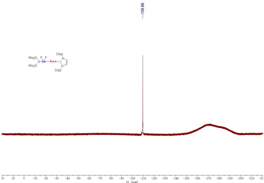
**Fig. S34**  $^{19}\text{F}$  NMR spectrum of **8** in  $\text{CDCl}_3$ .
