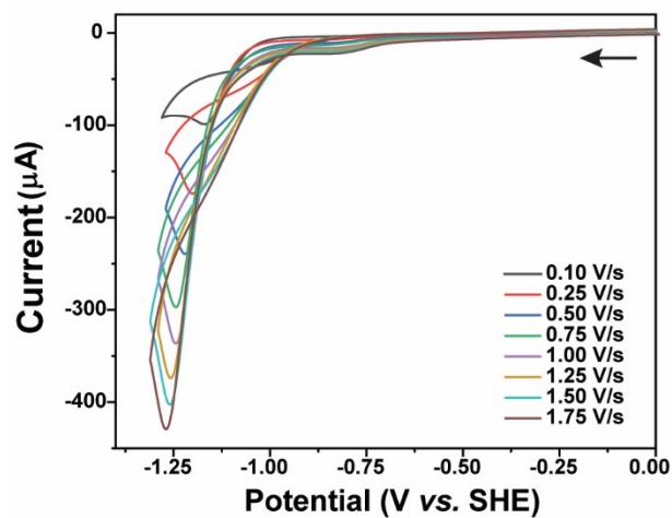
**Figure S12:** The cyclic voltammograms (CV) of complex C1 (0.25mM) at pH 5.0 under  $N_2$  at various scan rates. A 1 mm glassy carbon disc working electrode, Ag/AgCl reference electrode, and Pt-wire counter electrode were used along with  $Na_2SO_4$  as supporting electrolyte. The initial scan direction is displayed by the black arrows.
