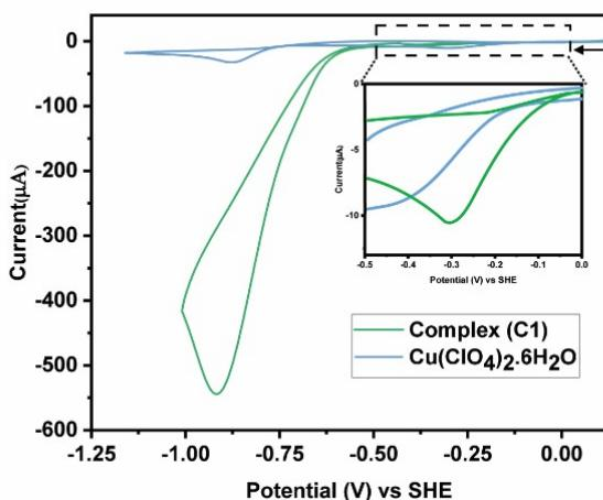
**Figure S24:** The comparative cyclic voltammetry data recorded for complex (0.5 mM) and  $\text{Cu}(\text{ClO}_4)_2 \cdot 6\text{H}_2\text{O}$  (0.5mM) at pH 2. The scan rate of 0.75 V/s were used during this experiment.
