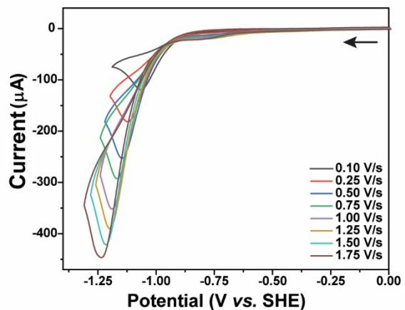
**Figure S14:** The cyclic voltammograms (CV) of complex C1 (0.25 mM) at pH 3.0 under  $\text{N}_2$  at various scan rates. A 1 mm glassy carbon disc working electrode, Ag/AgCl reference electrode, and Pt-wire counter electrode were used along with  $\text{Na}_2\text{SO}_4$  as a supporting electrolyte. The initial scan direction is displayed by the black arrows.
