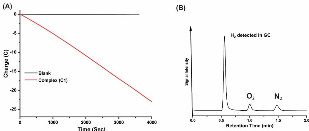
**Figure S9.** (A) Bulk electrolysis data recorded in DMF for 0.25 mM of **C1** (red trace) and blank DMF (Black Trace). Reticulated Vitreous Carbon was used as working electrode, Ag/AgCl as reference electrode and Coiled Pt-wire as counter electrode. (B) The Gas Chromatography data recorded after injecting 0.6 mL of head space gas using leur-lock gas-tight syringe after 4000 sec.
