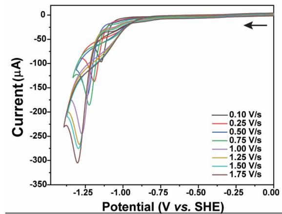
**Figure S11:** The cyclic voltammograms (CV) of complex **C1** (0.25 mM) at pH 6.0 under  $\text{N}_2$  at various scan rates. A 1 mm glassy carbon disc working electrode, Ag/AgCl reference electrode, and Pt-wire counter electrode were used along with  $\text{Na}_2\text{SO}_4$  as supporting electrolyte. The initial scan direction is displayed by the black arrows.
