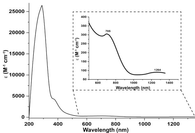
**Figure S5:** The optical spectra recorded for complex **C1** (black trace) in DMF expanding till 1350 nm at room temperature. The inset highlights the different bands originating from the  $d-d$  transition.
