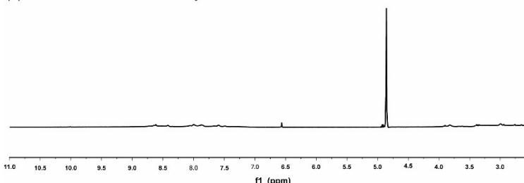
(B)  $^1\text{H}$  NMR of C1 after bulk electrolysis
