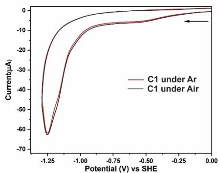
**Figure S20:** The comparative CV data recorded for complex **C1** at 1.25 V/s under Ar (red trace), and air (black trace).
