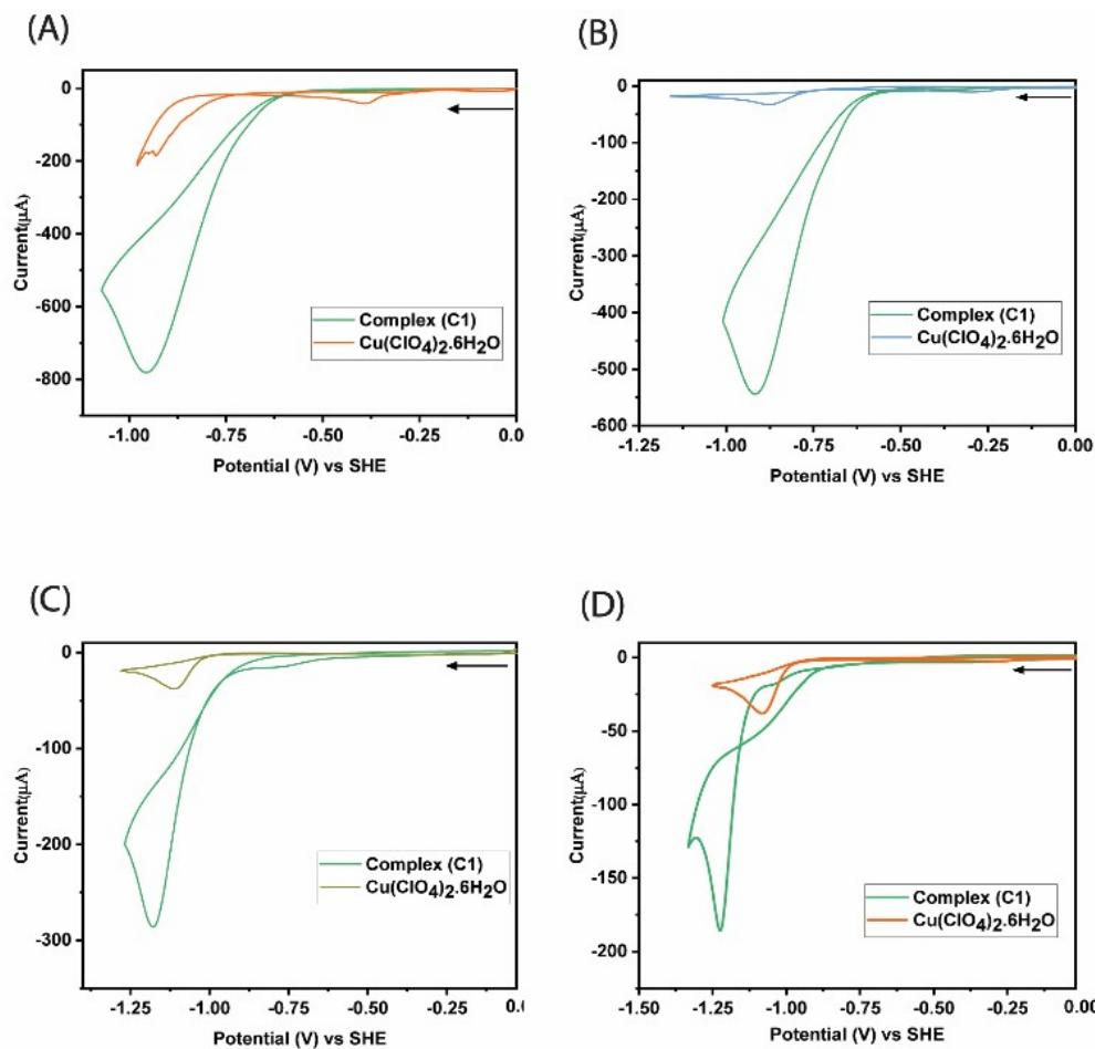
**Figure S23:** The comparative Cyclic Voltammetry data recorded for the complex (0.25 mM) and  $\text{Cu}(\text{ClO}_4)_2 \cdot 6\text{H}_2\text{O}$  (0.25mM) at various pH: (A) pH 1 (B) pH 2 (C) pH 4 (D) pH 6.
