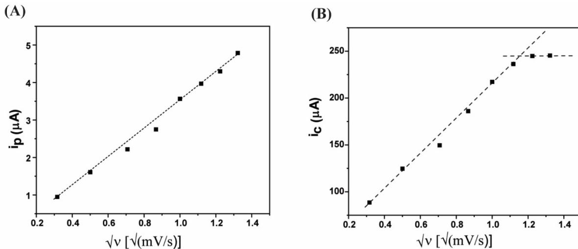
**Figure S17:** (A) Plot of current at -0.5 V vs. square root of scan rate recorded for **C1** at pH 6.0. The linear increase in the current with scan rate shows the stoichiometric nature of the signal. (B) Plot of current at -1.25 V vs. square root of scan rate recorded for **C1**. The non-linear variation at higher scan rate indicates the involvement of catalysis.
