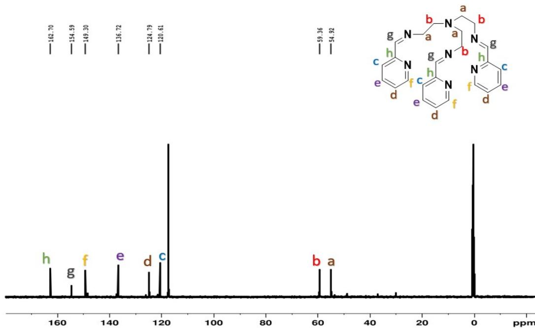
Figure S3. The  $^{13}\text{C}$ -NMR spectra for ligand **L1** recorded in  $\text{CD}_3\text{CN}$  solvent at room temperature.
