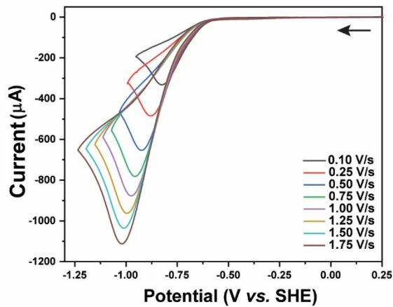
**Figure S16:** The cyclic voltammograms (CV) of complex **C1** (0.25mM) at pH 1.0 under  $\text{N}_2$  at various scan rates. (A), Here 1 mm glassy carbon disc working electrode, Ag/AgCl reference electrode, and Pt-wire counter electrode was used along with  $\text{Na}_2\text{SO}_4$  as a supporting electrolyte. The initial scan direction is displayed by the black arrows.
