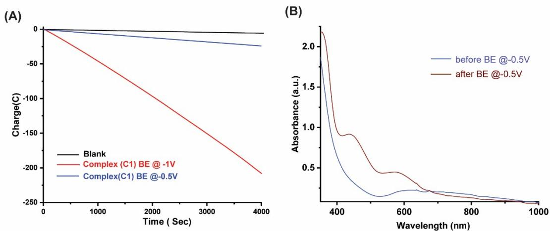
**Figure S25:** (A) The comparative Bulk electrolysis data recorded for **C1** at pH 1 at -0.5 V (vs. SHE) and -1 V (vs. SHE). (B). The comparative UV spectra before and after bulk electrolysis.
