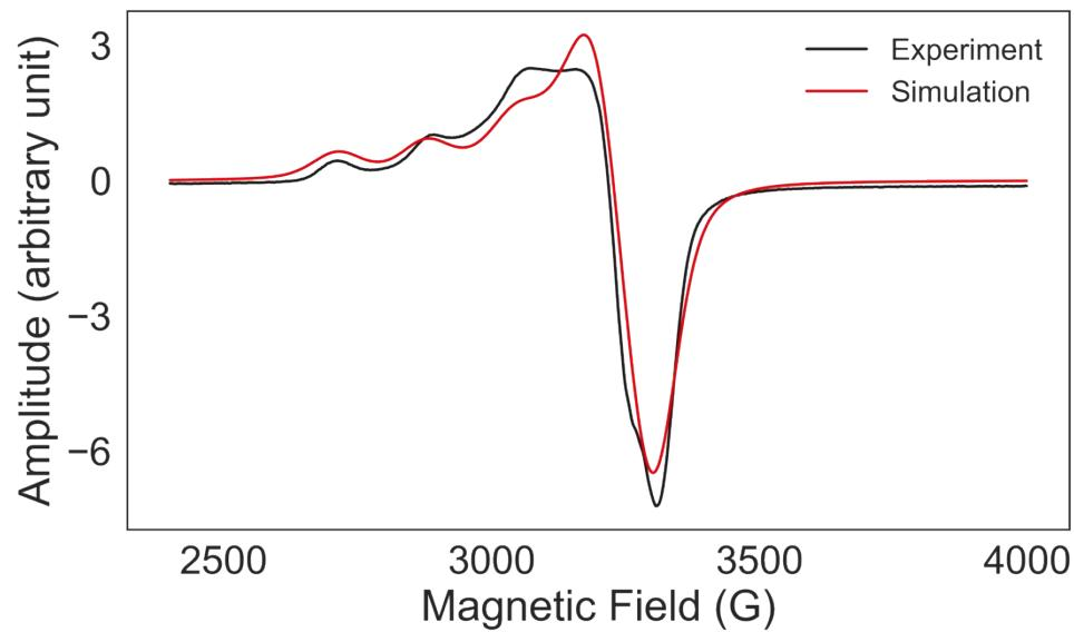
**Figure S7:** The experimentally observed (black trace) and simulated (red trace) EPR spectra for complex **C1** recorded at 100 K in DMF media.
