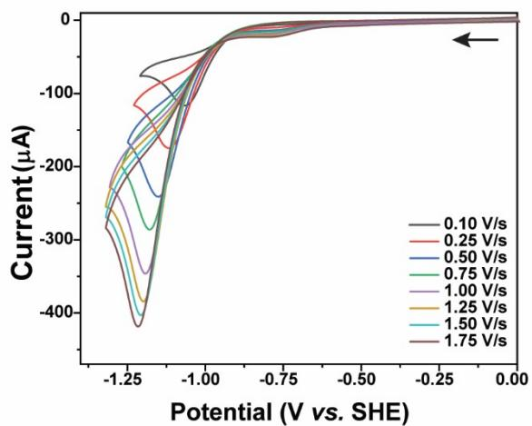
**Figure S13:** The cyclic voltammograms (CV) of complex C1 (0.25mM) at pH 4.0 under  $N_2$  at various scan rates. A 1 mm glassy carbon disc working electrode, Ag/AgCl reference electrode, and Pt-wire counter electrode were used along with  $Na_2SO_4$  as a supporting electrolyte. The initial scan direction is displayed by the black arrows.
