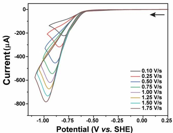
**Figure S15:** The cyclic voltammograms (CV) of complex C1 (0.25 mM) at pH 2.0 under  $\text{N}_2$  at various scan rates. A 1 mm glassy carbon disc working electrode, Ag/AgCl reference electrode, and Pt-wire counter electrode were used along with  $\text{Na}_2\text{SO}_4$  as a supporting electrolyte. The initial scan direction is displayed by the black arrows.
