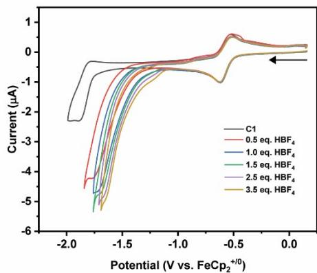
**Figure S10.** The CV data of **C1** (0.25mM) in analogous conditions with the serial addition of  $\text{HBF}_4$  where all the data were recorded at the scan rate of 1 V/s. Here 1mm glassy carbon disc working electrode, Ag/AgCl reference electrode, and Pt-wire counter electrode was used along with 0.1 M TBAF as a supporting electrolyte. The initial scan direction is displayed by the black arrows.
