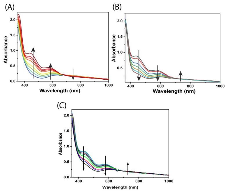
**Figure S18:** The gradual changes in the optical spectra of complex **C1** (0.2 mM) at pH 6.0 at room temperature: (A), potential of the solution held at -0.63 V vs. SHE; (B) potential held at -1.25 V vs. SHE; (C) potential held at -0.05V vs. SHE. A 3 mm glassy carbon rod, a Pt wire, and Ag/AgCl (in saturated KCl) were used as working electrode, counter electrode, and reference electrode, respectively, during the chronocoulometric experiment.
