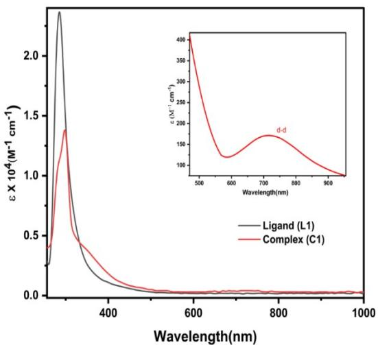
**Figure S4.** Comparative optical spectra recorded for ligand **L1** (black trace) and complex **C1** (red trace) in DMF exhibiting  $\pi-\pi^*$  and LMCT transitions at room temperature. The inset exhibits  $d-d$  transition recorded for **C1** under the same conditions.
