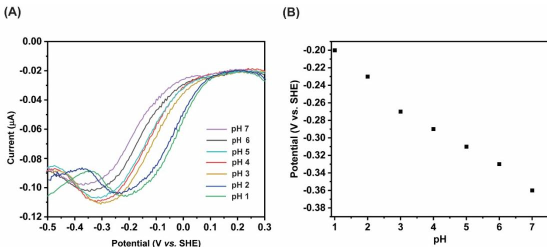
**Figure S21:** (A) The differential pulse voltammetry (DPV) data for **C1** (0.5mM) recorded at pH 1.0-7.0 (B) pH-dependency of the stoichiometric Cu(II/I) reduction potential for **C1** at different pH conditions ranging from pH 1.0 to pH 7.0.
