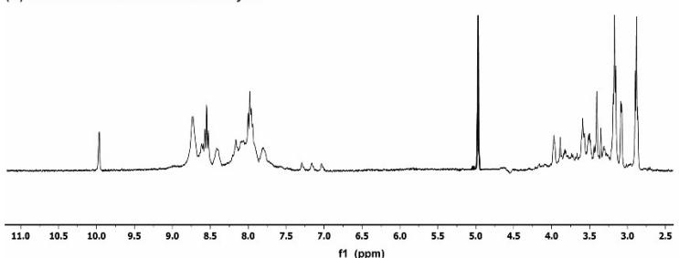
**Figure S31:** The  $^1\text{H}$  NMR data recorded for complex **C1** in  $\text{H}_2\text{O}$  blended  $\text{D}_2\text{O}$  solution ( $\text{pD} \sim 6.0$ ) (A) before and (B) after bulk electrolysis.
