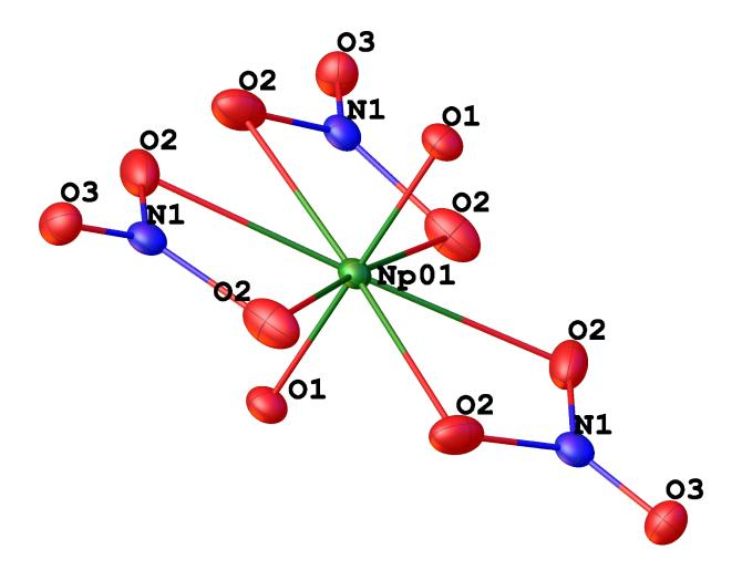
**Figure S1.** Crystal structure for (NH<sub>4</sub>)(NpO<sub>2</sub>)(NO3)<sub>3</sub> crystallized from feed solution. Major differences from the Autillo (2022) structure are a contracted unit cell with higher symmetry and the coordination of N2 along the neptunyl axis instead of off-axis nearer to O3. Hydrogen atoms are excluded from the ammonium atom (N2), as X-ray diffraction cannot reliably identify H in a structure.
