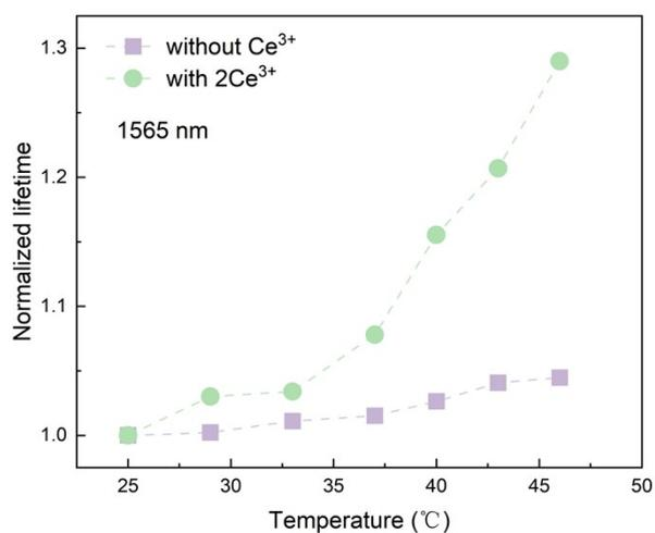
**Fig. S4.** Temperature-dependent luminescence decays of  $\text{NaYF}_4:5\text{Er}^{3+}/2\text{Ce}^{3+}@\text{NaYbF}_4@\text{NaYF}_4:40\text{Nd}^{3+}/20\text{Yb}^{3+}$  and  $\text{NaYF}_4:5\text{Er}^{3+}@\text{NaYbF}_4@\text{NaYF}_4:40\text{Nd}^{3+}/20\text{Yb}^{3+}$  nanoparticles dispersed in deionized water. Excitation at 808 nm, emission at 1565 nm.
