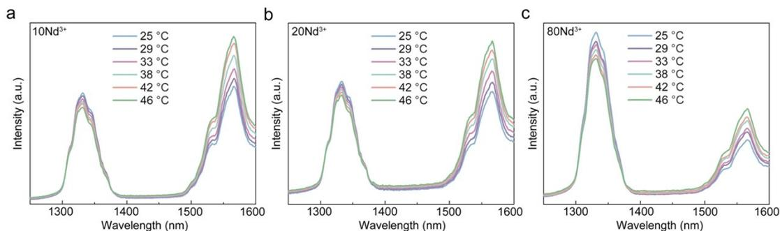
**Fig. S6.** Temperature-dependent emission spectra of the  $\text{NaYF}_4:5\text{Er}^{3+}/2\text{Ce}^{3+}@\text{NaYbF}_4@\text{NaYF}_4:\text{yNd}^{3+}/20\text{Yb}^{3+}$  nanocrystals: (a)  $10\text{Nd}^{3+}$ , (b)  $20\text{Nd}^{3+}$  and (c)  $80\text{Nd}^{3+}$ .
