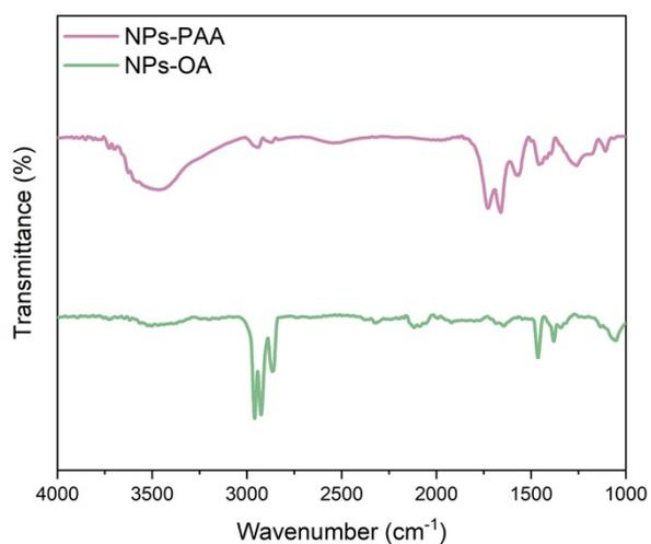
**Fig. S2.** FT-IR spectra of OA-capped and PAA-capped NPs.
