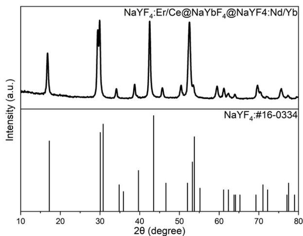
**Fig. S1.** X-ray diffraction pattern of the NaYF<sub>4</sub>:Er<sup>3+</sup>/Ce<sup>3+</sup>@NaYbF<sub>4</sub>@NaYF<sub>4</sub>:Nd<sup>3+</sup>/Yb<sup>3+</sup> nanoparticles and PDF card no.16-0334.
