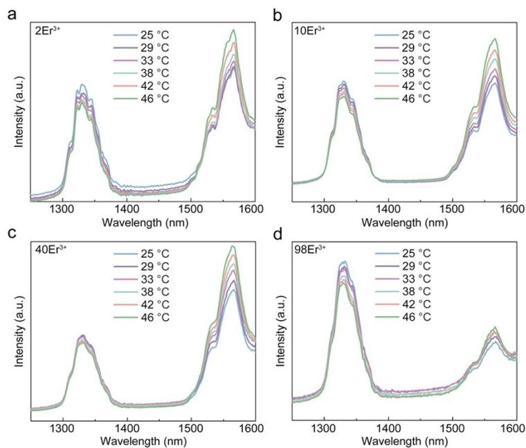
**Fig. S5.** Temperature-dependent emission spectra of the  $\text{NaYF}_4:\text{xEr}^{3+}/2\text{Ce}^{3+}@\text{NaYbF}_4@\text{NaYF}_4:40\text{Nd}^{3+}/20\text{Yb}^{3+}$  nanocrystals: (a)  $2\text{Er}^{3+}$ , (b)  $10\text{Er}^{3+}$ , (c)  $40\text{Er}^{3+}$  and (d)  $98\text{Er}^{3+}$ .
