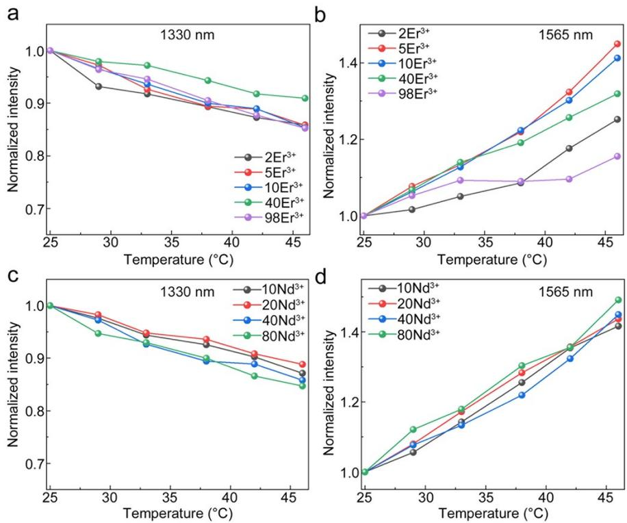
**Fig. S8.** Normalized 1330 emission intensity against the temperature with varying (a)  $\text{Er}^{3+}$  doping concentrations, and (c)  $\text{Nd}^{3+}$  doping concentrations. Normalized 1565 nm emission intensity against the temperature with varying (b)  $\text{Er}^{3+}$  doping concentrations, and (d)  $\text{Nd}^{3+}$  doping concentrations.
