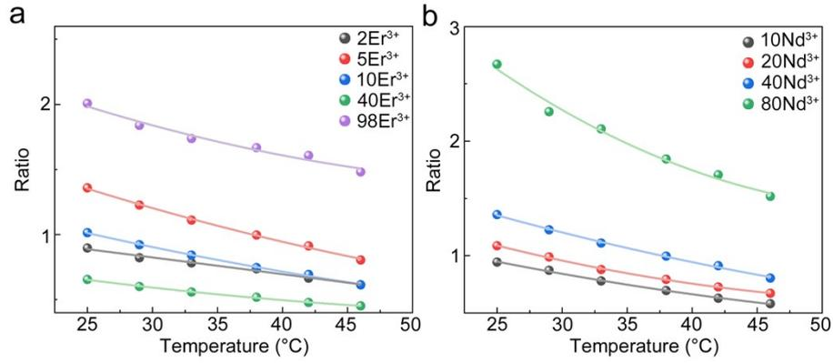
**Fig. S7.** The change in  $R$  with temperature for nanoparticles with different (a)  $\text{Er}^{3+}$  doping concentrations and (b)  $\text{Nd}^{3+}$  doping concentrations.
