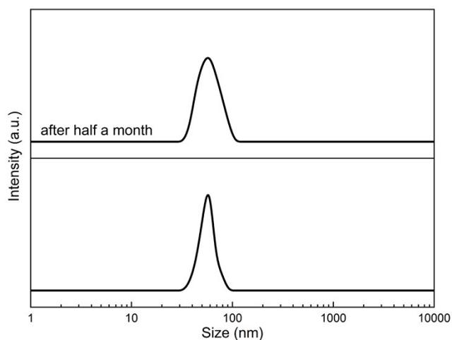
**Fig. S3.** Dynamic light scattering (DLS) size distribution of NPs (a) dissolved in phosphate-buffered saline (PBS) and (b) after storage for half a month.
