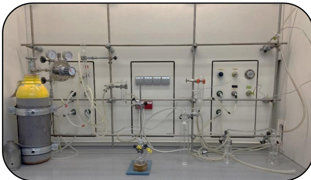
**Figure S1.** Setup for the preparation of  $\text{NH}_3$  solutions in organic solvents.
