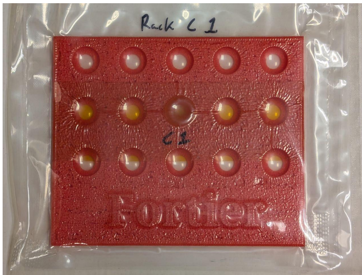
Fig. S6 Photograph of a wax coin fitted within a 3D-printed sample rack (160 mm × 145 mm × 7 mm), vacuum sealed within food-grade EVOH and poly-nylon films.
