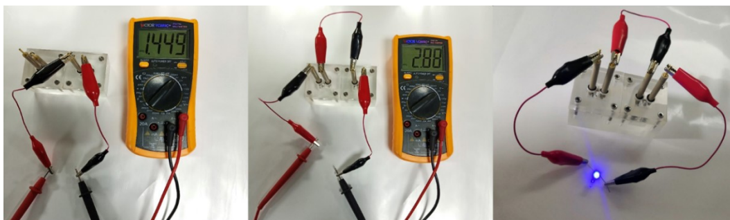
Fig. S14 The photograph of a blue, green and red LED powered by two tandem ZABs.
