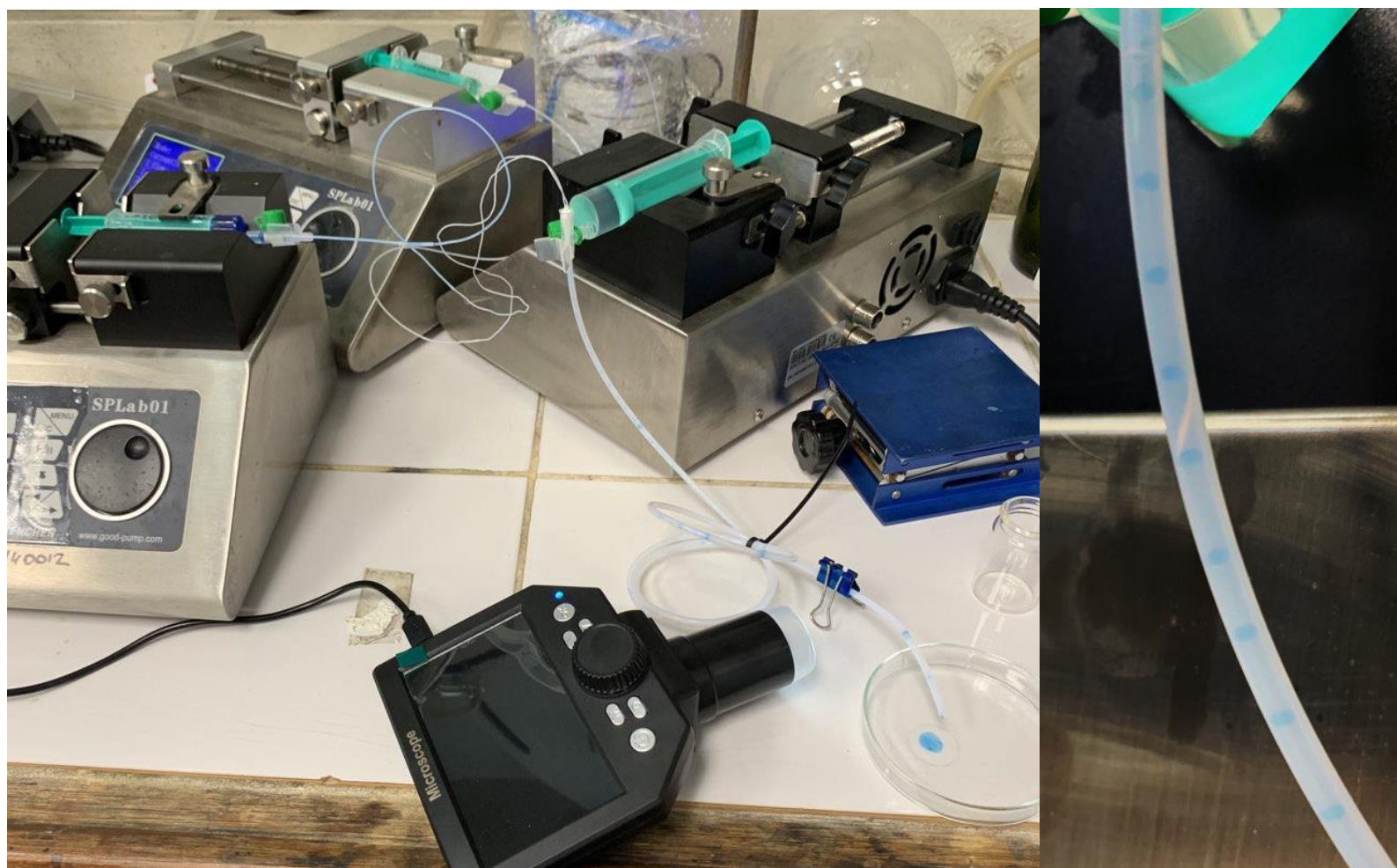
Figure S10.5. Set-up and droplets formed in optimal conditions
