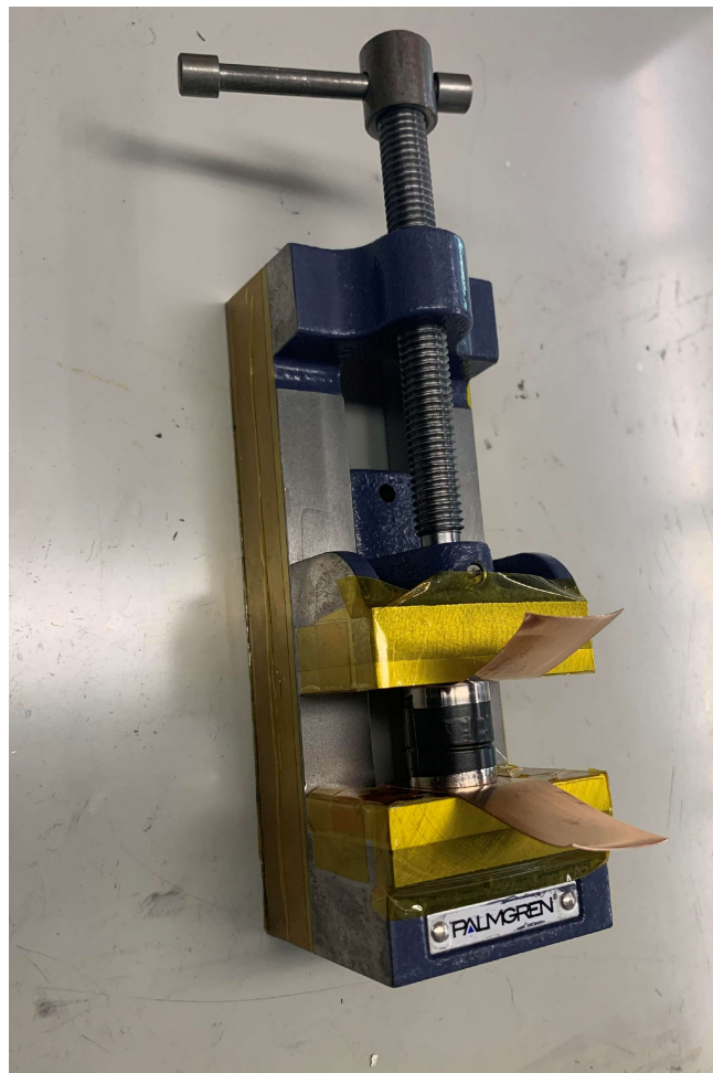
Figure S1. Electrochemical impedance spectroscopy cell setup. Kapton-covered vise sandwiches two copper strips and the EIS pellet cell (sealed with electrical tape) to retain contact and constant pressure.
