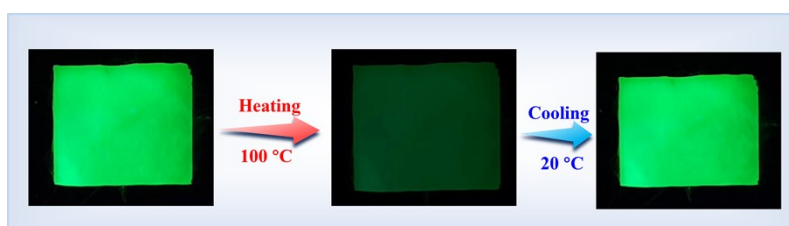
Fig. S17. Physical photos of CsPbX 3 -UCLNPs/PS film after a heating/cooling cycle process under UV light
