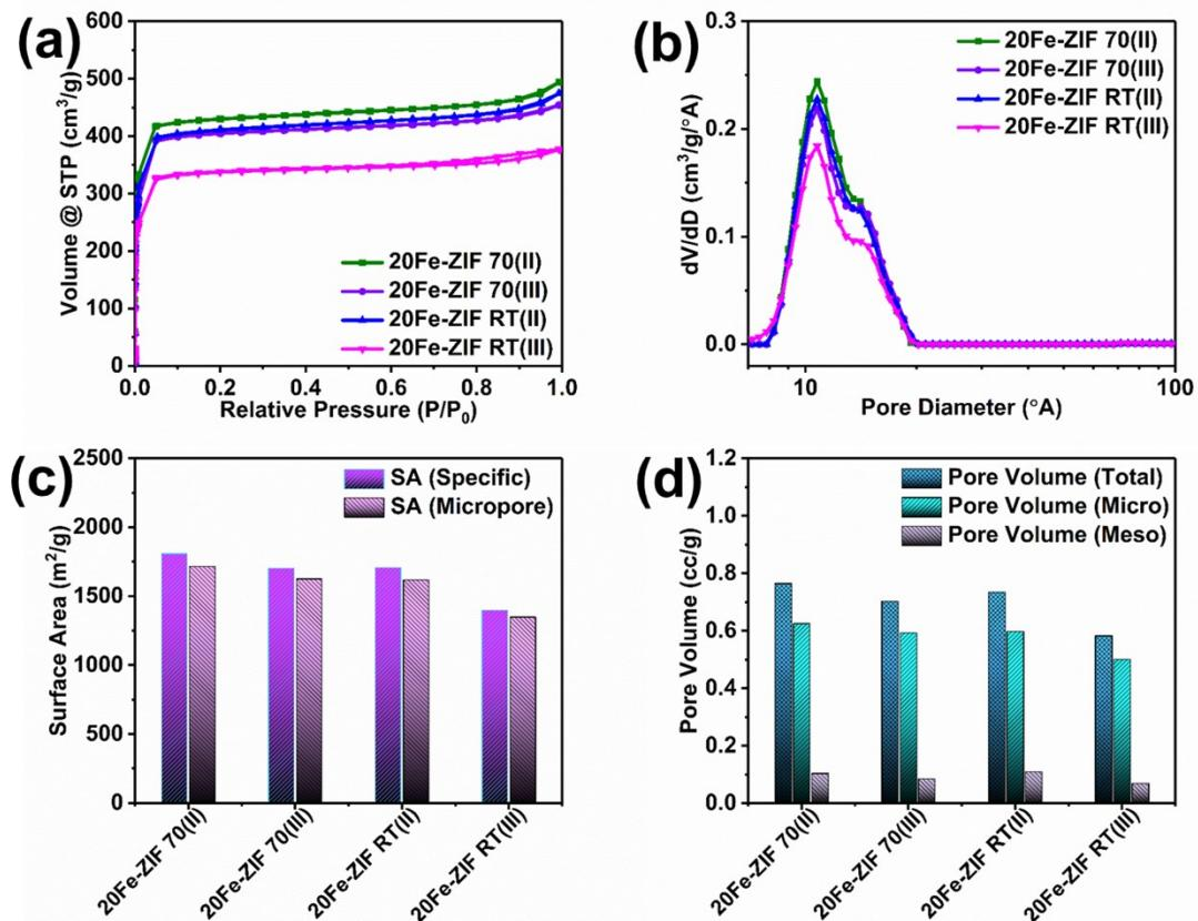
**Fig. S9** (a)  $N_2$  adsorption-desorption isotherms and (b) Pore size distribution (c) Surface area and (d) Pore volume of the 20Fe-ZIF precursors.
