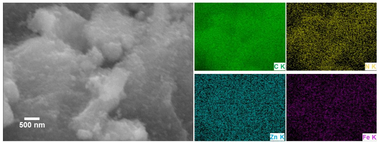
**Fig. S4** (a) FESEM image, (b) Corresponding EDX elemental mapping of 20Fe-N-C RT(III).
