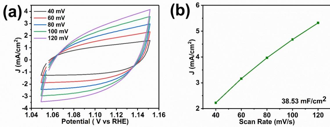
**Fig. S18** Representative double-layer capacitance measurements of 20Fe-N-C 70(II) showing (a) CV curves and (b) capacitive current against the scan rates.
