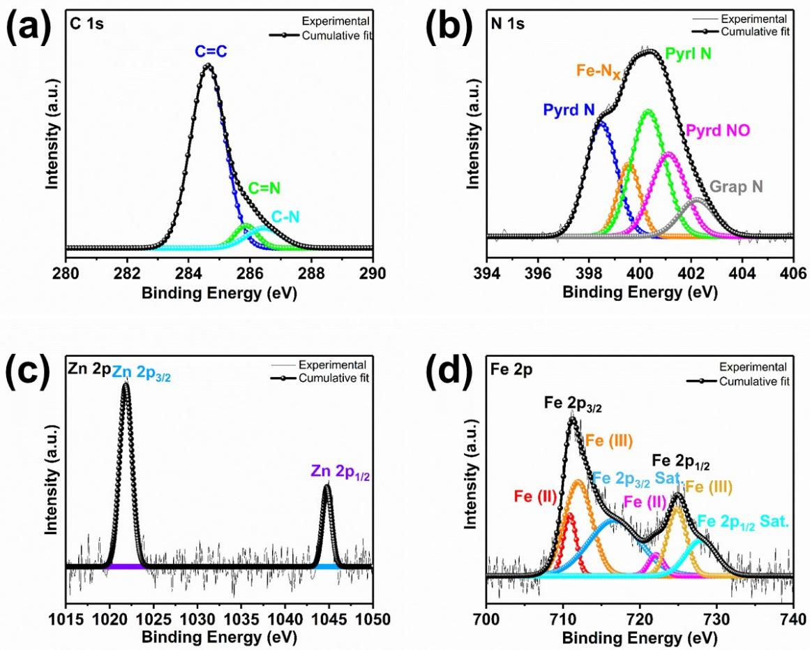
**Fig. S12** High resolution XPS spectra of (a) C 1s (b) N 1s (c) Zn 2p and (d) Fe 2p in 20Fe-N-C 70(II) catalyst.
