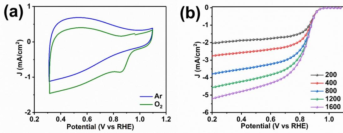
**Fig. S16** (a) CV and (b) LSV curves of 20Fe-N-C RT(III) in 0.1M KOH.
