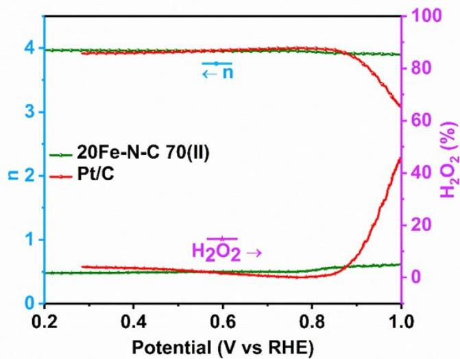
**Fig. S24** RRDE result of the catalysts in 0.5M  $\text{H}_2\text{SO}_4$
