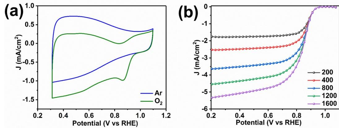
**Fig. S17** (a) CV and (b) LSV curves of 20Fe-N-C 70(III) in 0.1M KOH.
