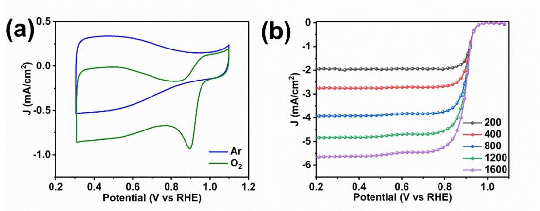
**Fig. S15** (a) CV and (b) LSV curves of 20Fe-N-C RT(II) in 0.1M KOH.
