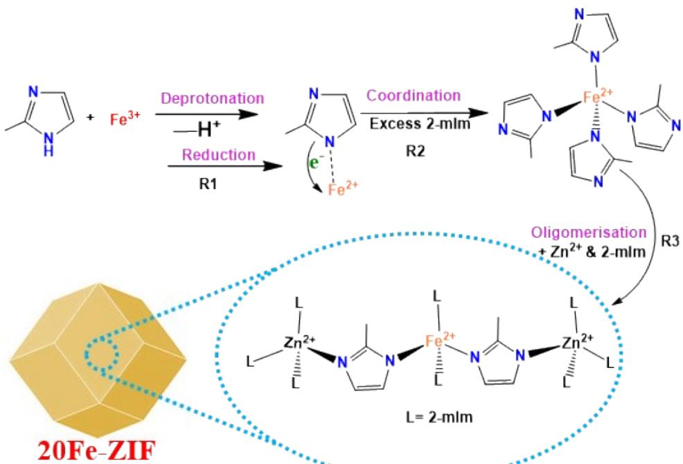
**Fig. S10** Proposed mechanism of in-situ  $\text{Fe}^{3+}$  reduction during the synthesis of 20Fe-ZIF (III) precursors.
