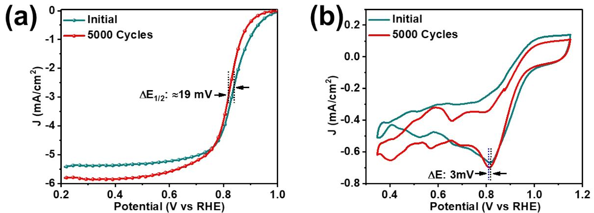
**Fig. S21** (a) LSV and (b) CV curves of Pt/C before and after the accelerated stress test.
