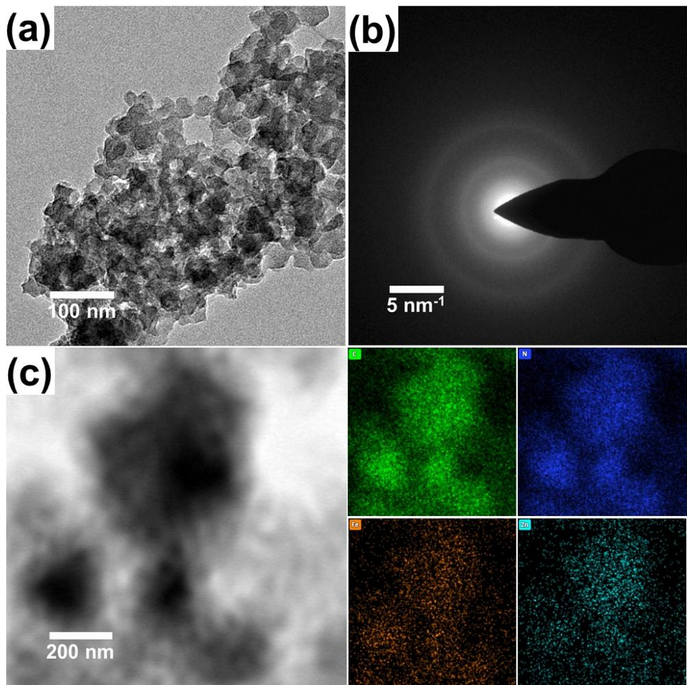
**Fig. S22** (a) STEM image (b) SAED pattern (c) BF-STEM image with corresponding EDS elemental mapping result of 20Fe-N-C 70(II) after 5000 cycles of potential stress test.
