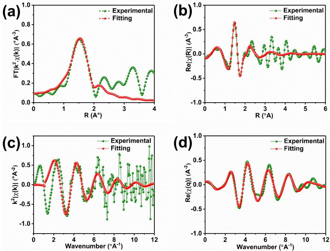
**Fig. S13** Fitting results of FT-EXAFS spectra of 20Fe-N-C 70(II) in (a)-(b) R space and (c)-(d) k-space.
