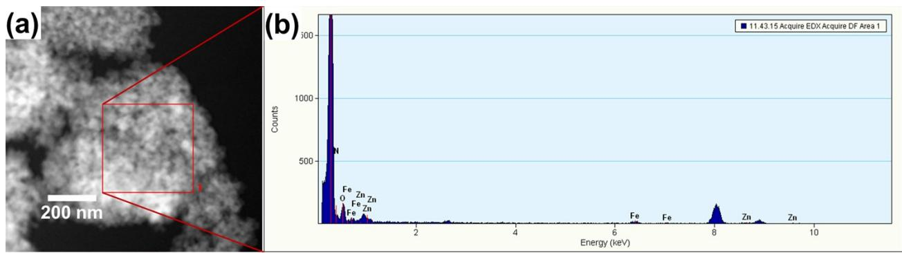
**Fig. S8** (a) STEM image with (b) Corresponding EDX spectrum of 20Fe-N-C 70(II).
