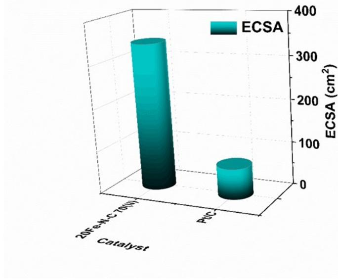
**Fig. S19** Typical ECSA of the catalysts.
