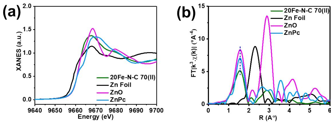
**Fig. S14** (a) XANES and (b) FT-EXAFS spectra of 20Fe-N-C 70(II) and reference standards at Zn K-edge.
