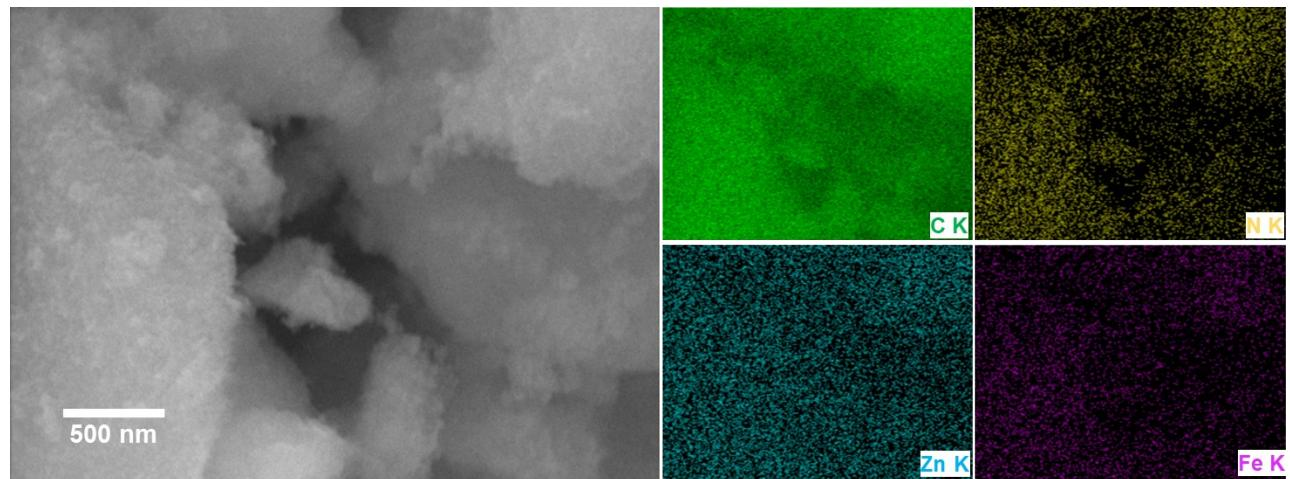
**Fig. S3** (a) FESEM image, (b) Corresponding EDX elemental mapping of 20Fe-N-C RT(II).
