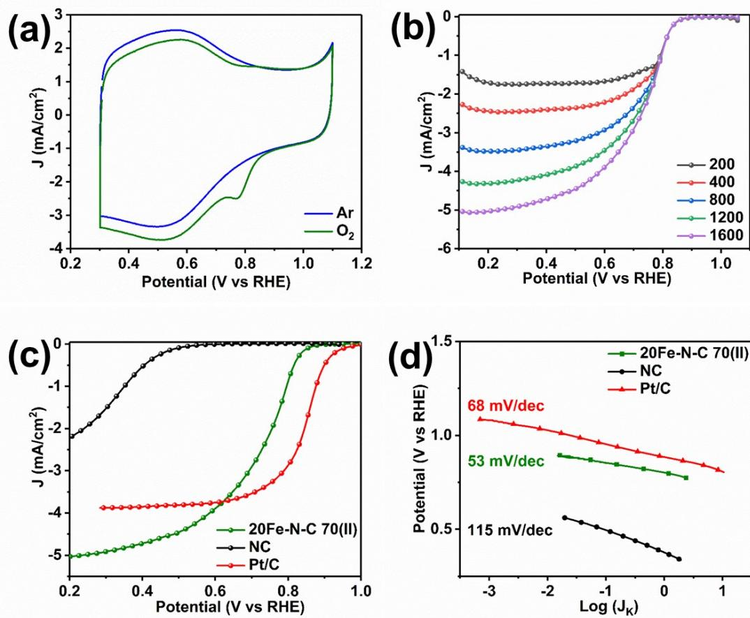
**Fig. S23** (a) Electrochemical ORR activity of the catalysts in 0.5M  $\text{H}_2\text{SO}_4$  with 800  $\mu\text{g}/\text{cm}^2$  loading showing (a) CV and (b) LSV curves of 20Fe-N-C 70(II), (c) LSV curves and (d) Tafel slopes of the catalysts. (Pt/C loading: 40  $\mu\text{g}_{\text{Pt}}/\text{cm}^2$ )
