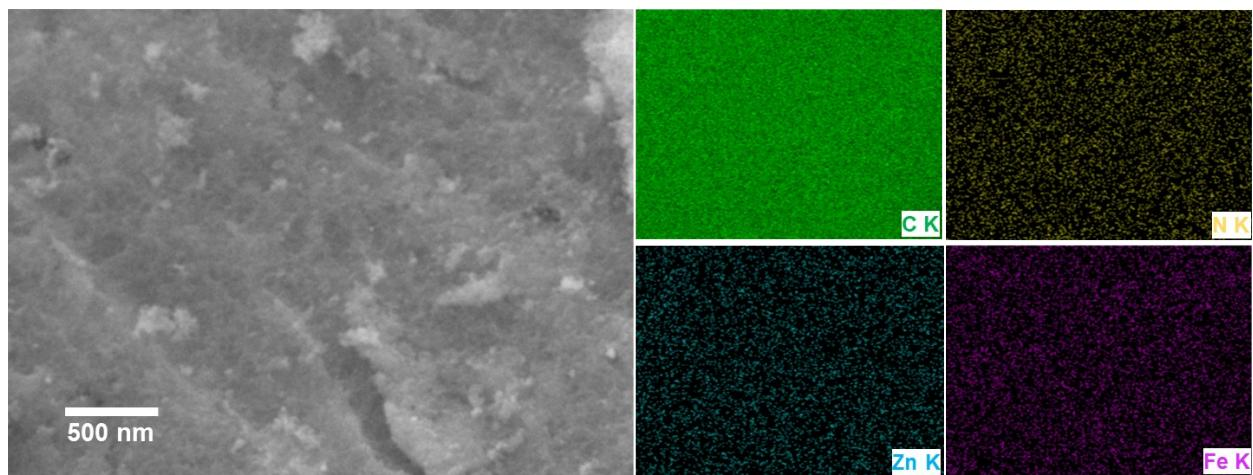
**Fig. S6** (a) FESEM image, (b) Corresponding EDX elemental mapping of 20Fe-N-C 70(III).
