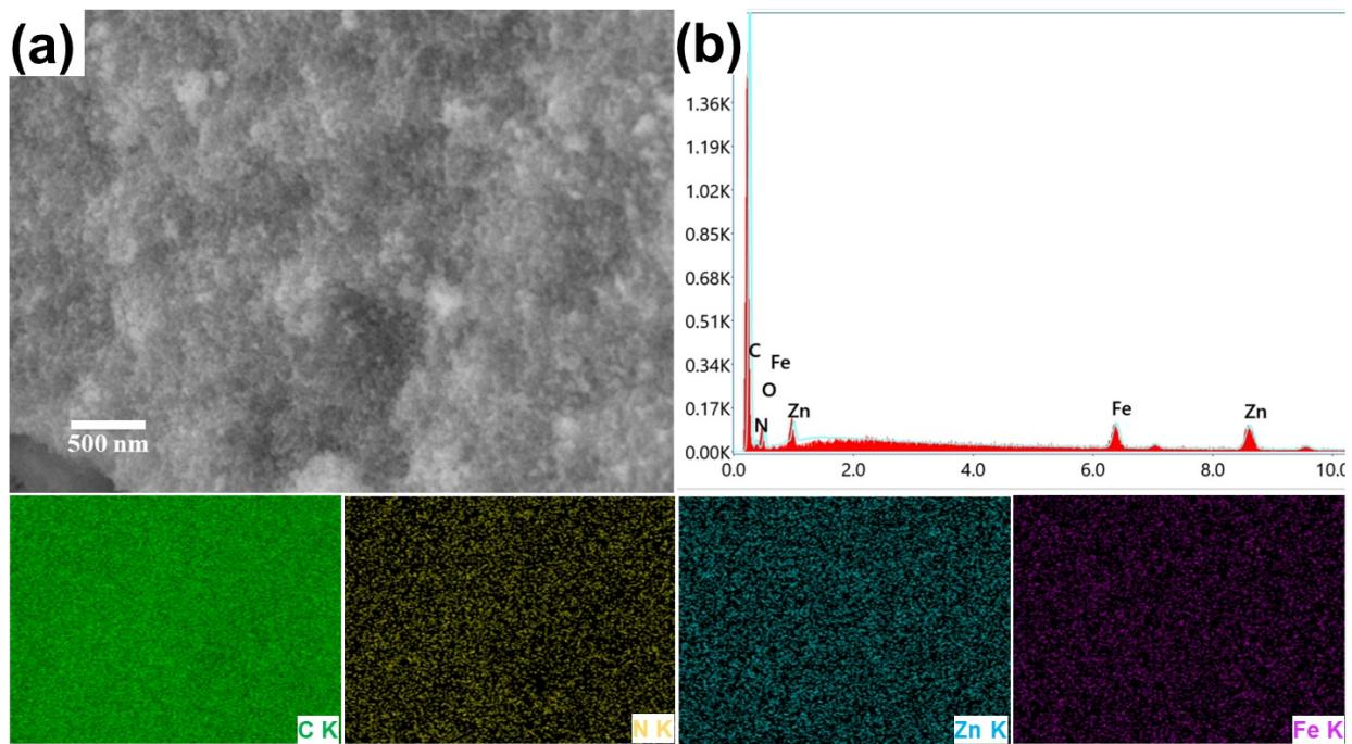
**Fig. S5** (a) FESEM image, (b) EDX pattern of 20Fe-N-C-70(II) with corresponding EDX elemental mapping.
