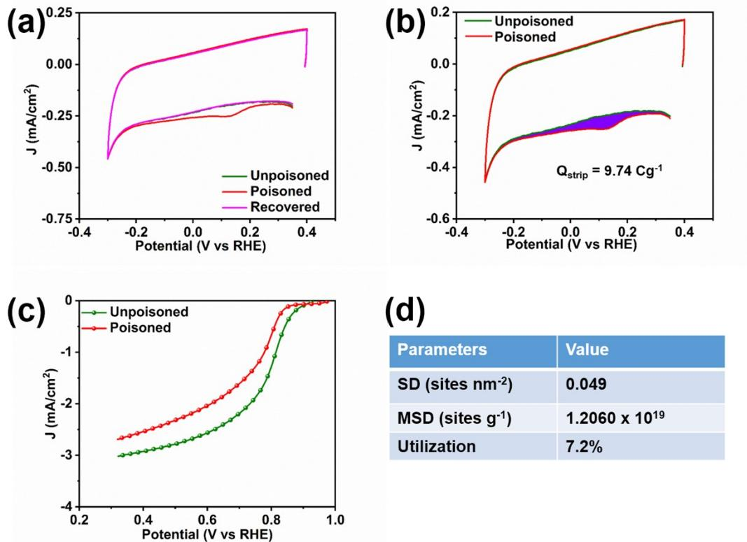
**Fig. S25** Site density evaluation of 20Fe-N-C 70(II) showing (a) Nitrite stripping voltammetry in  $\text{N}_2$ -saturated 0.5 M acetate electrolyte buffer (pH 5.2) before, during and after nitrite adsorption (b) CV curves in the reductive stripping region (c) ORR performance of catalyst layer before and after nitrite adsorption (d) SD calculation.
