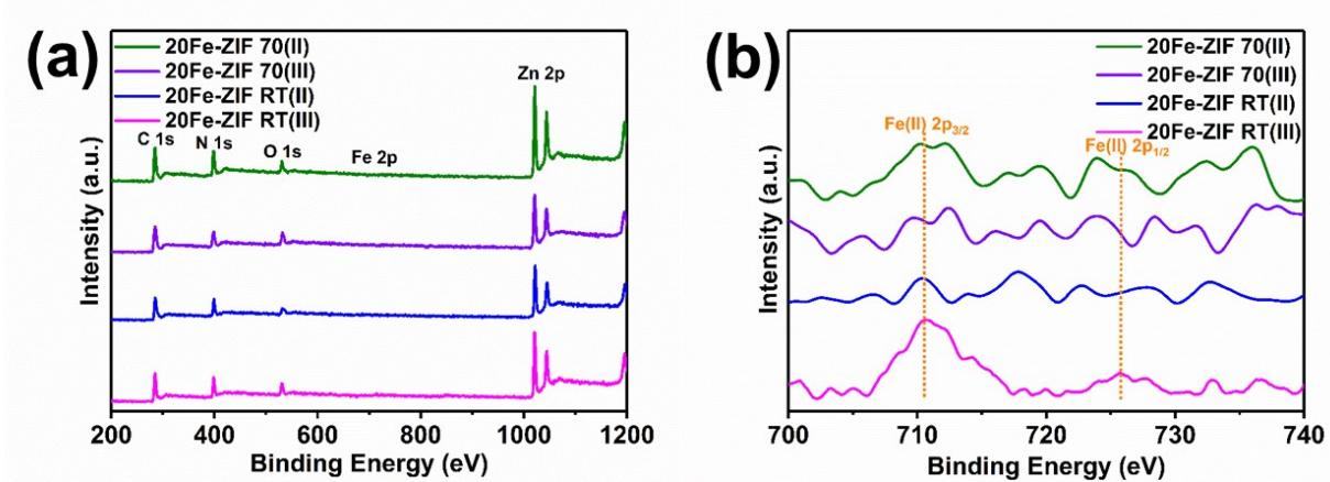
**Fig. S11** (a) XPS survey spectra and (b) High resolution XPS spectra of Fe 2p in 20Fe-ZIF precursors.
