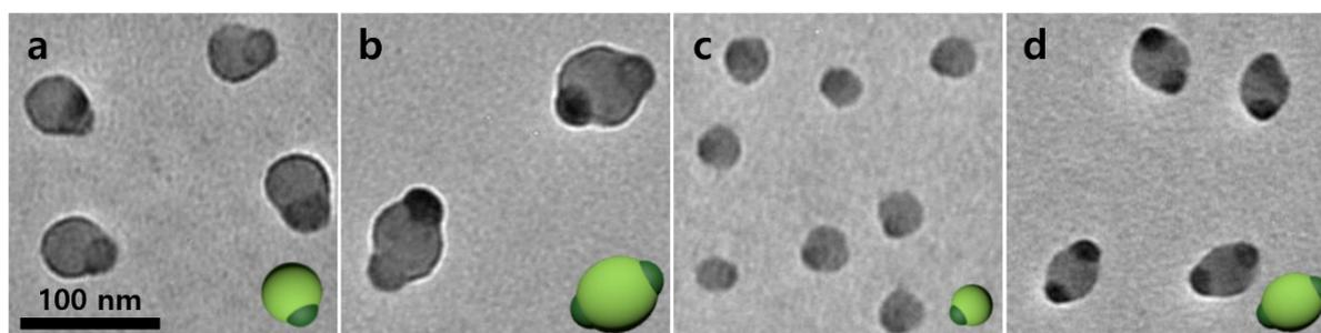
**Figure S8.** TEM images: (a) single-patch micelles of PS(266k)-*b*-P4VP(58k); (b) dimers of single-patch micelles of PS(266k)-*b*-P4VP(58k); (c) single-patch micelles of PS(80k)-*b*-P4VP(16k); (d) dimers of single-patch micelles of PS(80k)-*b*-P4VP(16k).
