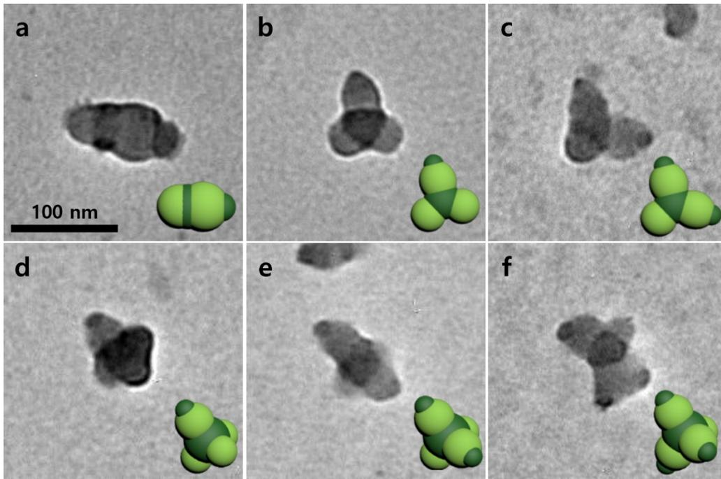
**Figure S9.** TEM images of patchy micelles partially assembled with single-patch micelles: (a) a two-patch micelle with one single-patch micelle; (b) a three-patch micelle with one single-patch micelle; (c) a three-patch micelle with two single-patch micelles; (d) a four-patch micelle with one single-patch micelle; (e) a four-patch micelle with two single-patch micelles; (f) a four-patch micelle with three single-patch micelles.
