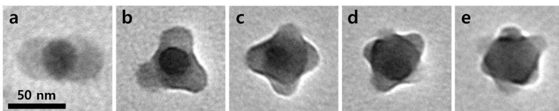
**Figure S5.** TEM images of patchy micelles after selective core staining with I<sub>2</sub>: (a) S2VP-2; (b) S2VP-3; (c) S2VP-4; (d) S2VP-5; (e) S2VP-6.
