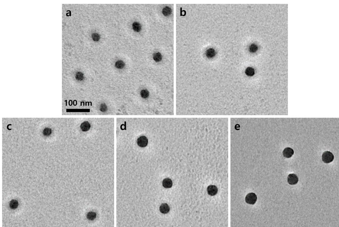
**Figure S4.** TEM images of S2VP micelles after staining the cores with  $I_2$ : (a) S2VP-2; (b) S2VP-3; (c) S2VP-4; (d) S2VP-5; (e) S2VP-6.
