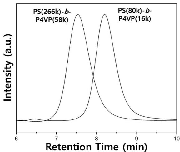
**Figure S6.** GPC profiles for PS-*b*-P4VP.
