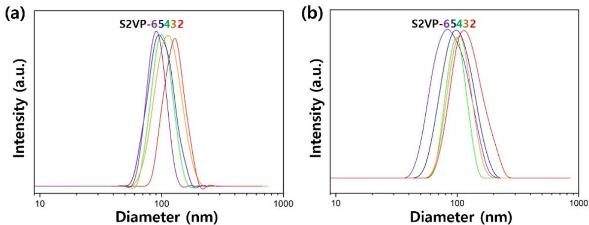
**Figure S3.** DLS results: (a) spherical micelles; (b) micelles with patches in polyhedral configurations.
