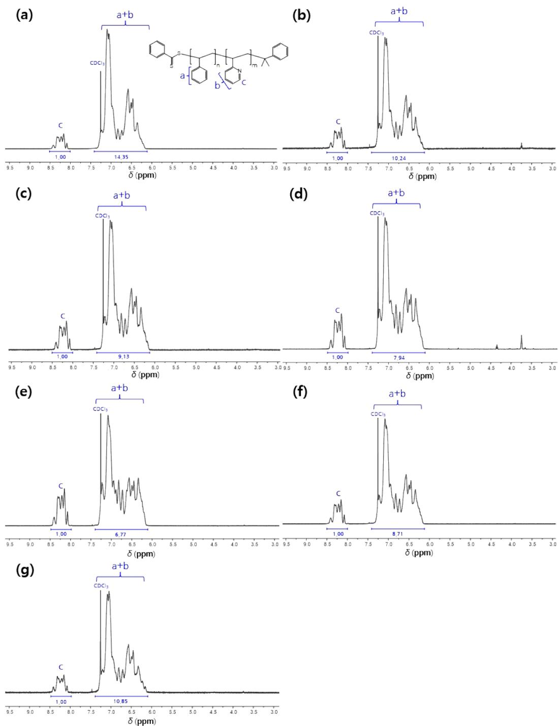
**Figure S2.** NMR spectra of PS-*b*-P2VP (S2VP): (a) S2VP-2; (b) S2VP-3; (c) S2VP-4; (d) S2VP-5; (e) S2VP-6; (f) S2VP-4s; (g) S2VP-4ss.
