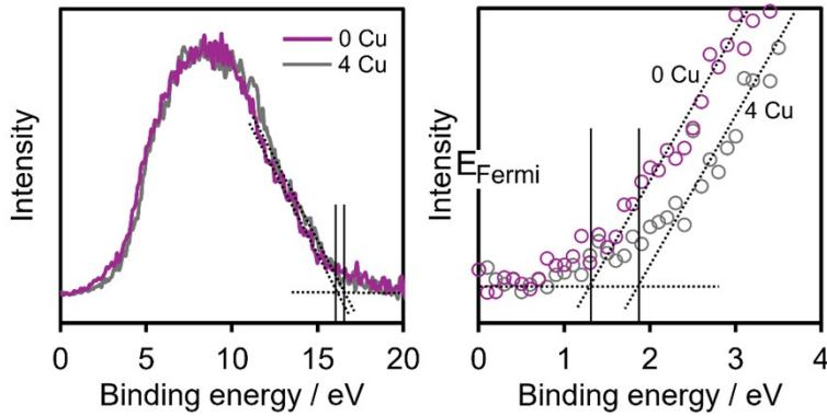
**Figure S6.** UPS spectra of gCN and 4Cu-gCN. The left figure shows photoelectron signal plotted with respect to the Fermi level at 0 eV and showing determination of the secondary electron cut-off (SECO). The right figure shows the region near the Fermi level, showing the determination of the VB edge.
