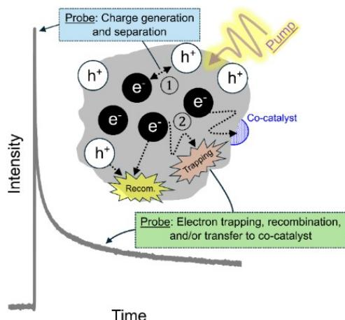
**Figure S5.** Schematic of the different photophysical phenomena that can be probed by TRMC.
