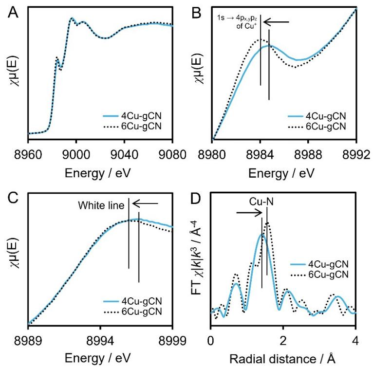
**Figure S1.** XANES spectra showing (A) the overall features, (B) the feature corresponding to Cu 1s  $\rightarrow$  4p transitions, and (C) a weak feature just after the absorption edge (white line). (D) FT-EXAFS spectra for the Cu-N coordination in R space.
