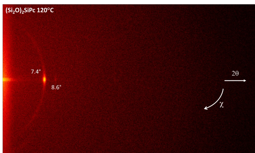
Figure S15: 2D-PXRD map of (Si 2 O) 2 SiPc thin film on ODTS-treated SiO 2 surfaces annealed at 120°C. The map ranges from 2\theta = 3^\circ to 30^\circ on the Y-axis, from the left to the right.
