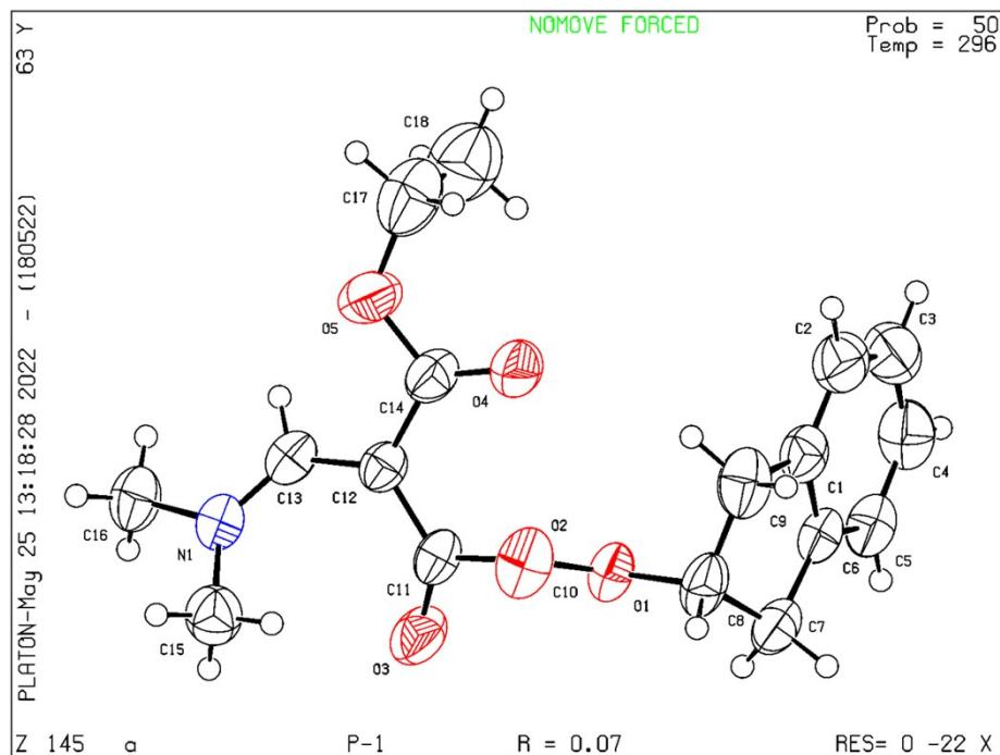
**Figure S2** ORTEP diagram of **3q** with thermal displacement parameters drawn at 50% probability.
