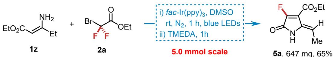
A 100 mL oven-dried reaction vessel equipped with a magnetic stirrer bar was charged with ethyl (Z)-3-aminopent-2-enoate **1z** (715 mg, 5 mmol), bromodifluoroacetate **2a** (2030 mg, 10 mmol), *fac*-Ir(ppy)<sub>3</sub> (16.38 mg, 0.025 mmol, 0.5 mol%) and dimethyl sulfoxide (DMSO, 50 mL). The reaction vessel was exposed to blue LEDs irradiation at room temperature in N<sub>2</sub> with stirring for 1 h. After
