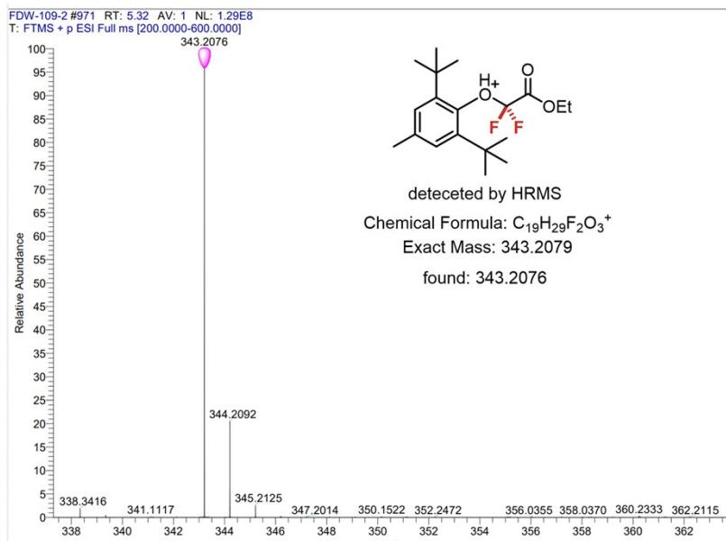
**Figure S4.** Radical trapping experiments
