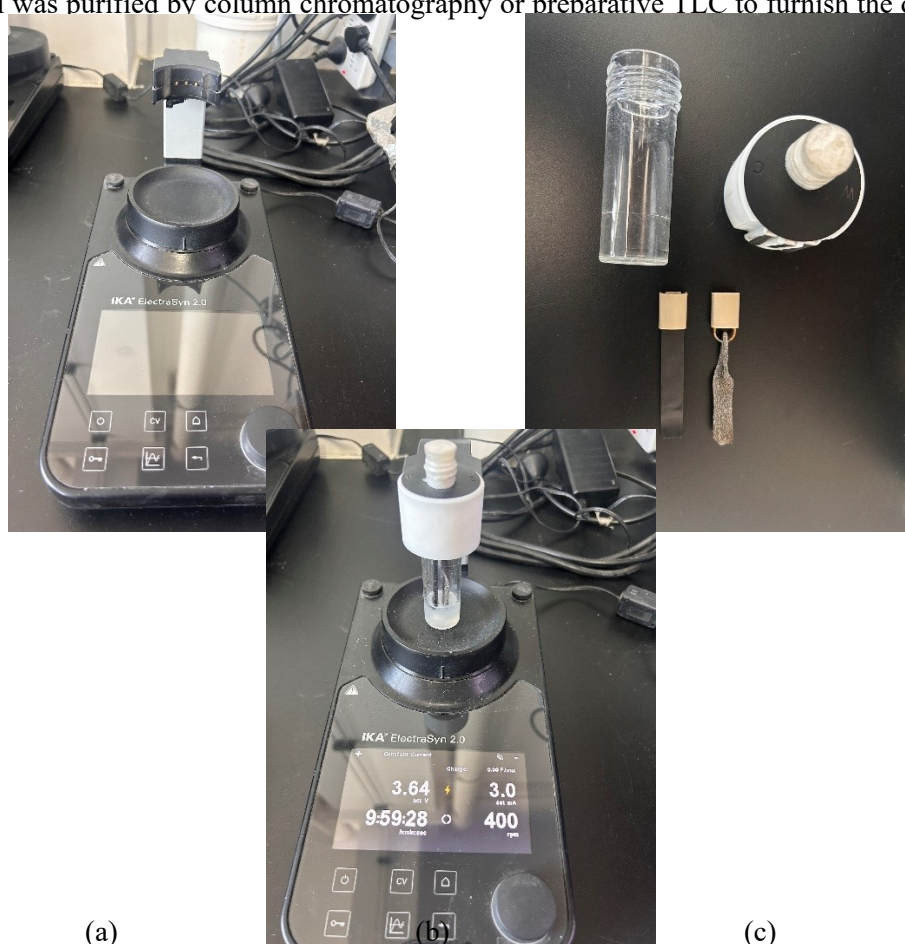
Figure S1. Electrocatalytic equipment. (a) IKA® ElectraSyn 2.0; (b) Electrodes and reaction vial; (c) Constant current power supply.
