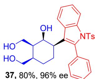
**((1R, 2S, 3S, 4R)-3-Hydroxy-4-(2-phenyl-1-tosyl-1H-indol-3-yl)cyclohexane-1, 2-diyl)dimethanol.**
