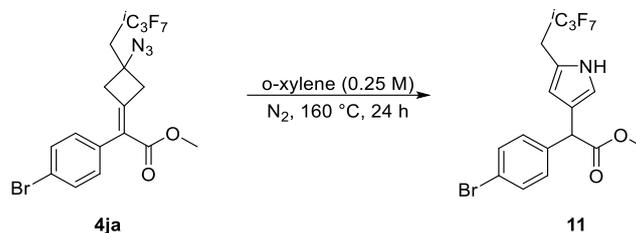
In a flame-dried Schlenk tube, the azide **4ja** (0.2 mmol, 1.0 equiv) was dissolved in o-xylene and stirred at 160 °C for 24 h. After completion, the organic solvent was evaporated under reduced pressure and the residue was purified by flash column chromatography on silica gel to afford the corresponding product as colorless oil (74 mg, 78% yield).
