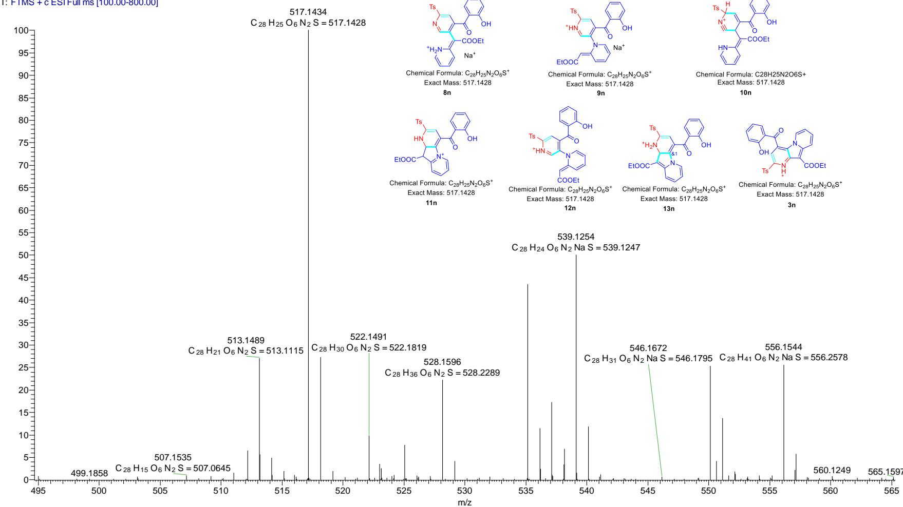
Figure S56. HRMs spectra of intermediates **8n/9n/10n/11n/12n/13n** and target compound **3n**
