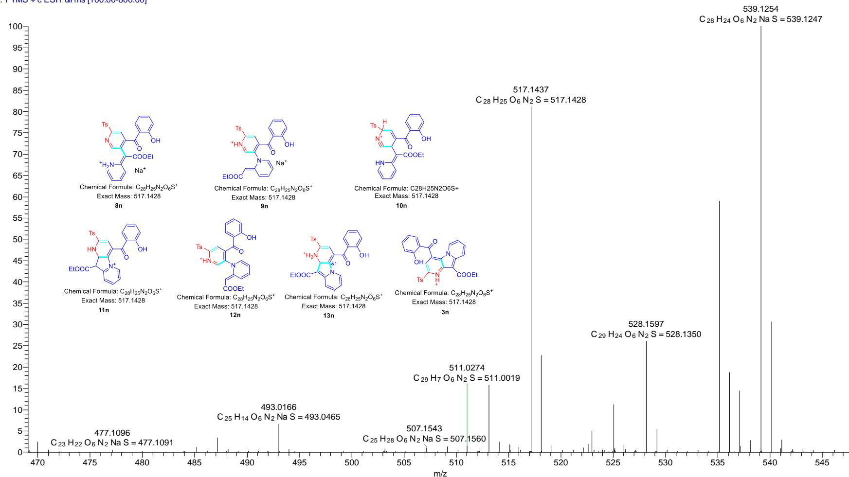
**Figure S57.** HRMs spectra of intermediates **8n/9n/10n/11n/12n/13n** and target compound **3n**
