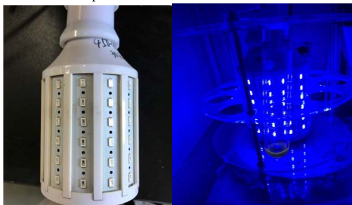
Figure S1. Photoreactor used in this work (30 W 450-460 nm blue LEDs, \lambda_{\text{max}} = 454 nm).
