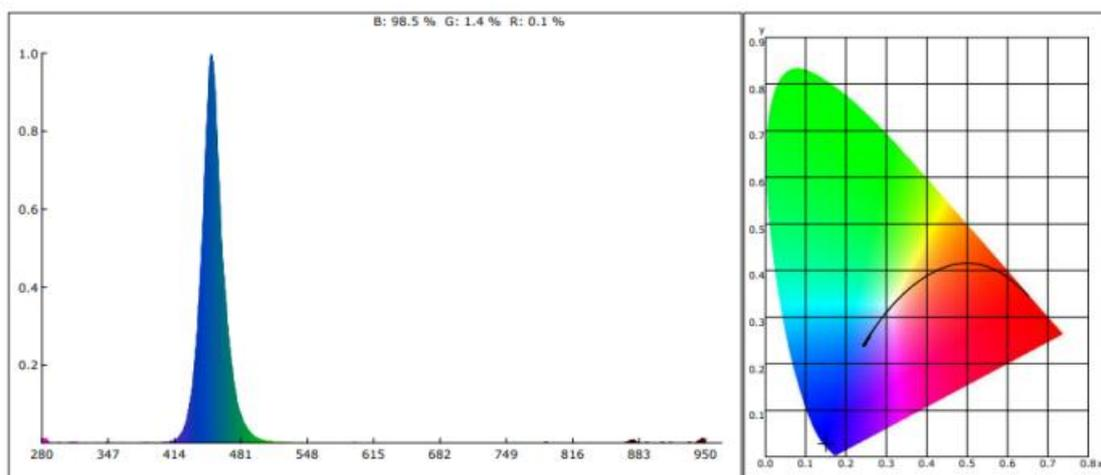
**Figure S2.** The spectrum of Blue LED
