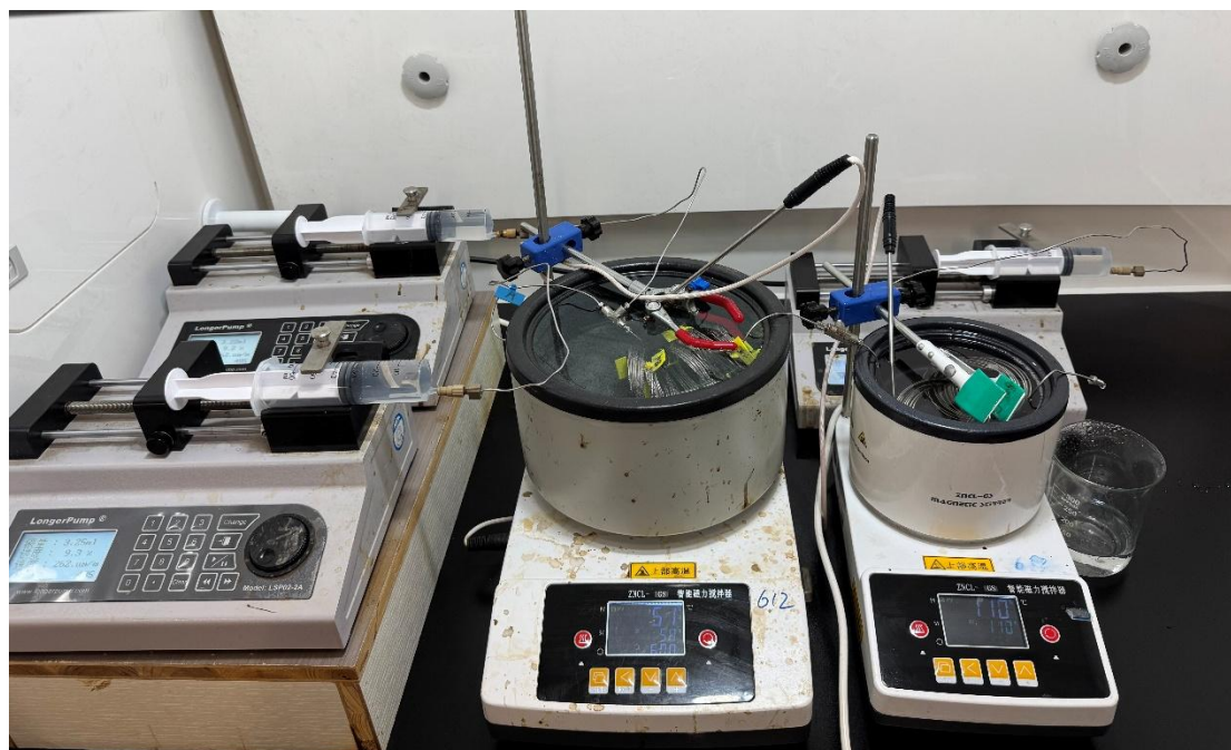
Fig. S1 Photographic representation of reaction equipment of two-step continuous flow telescoped synthesis of benzimidazoles.
