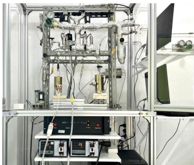
Figure S2. Schematic diagram (A) and photo (B) of pressure-composition-isotherm (PCI) test station.
