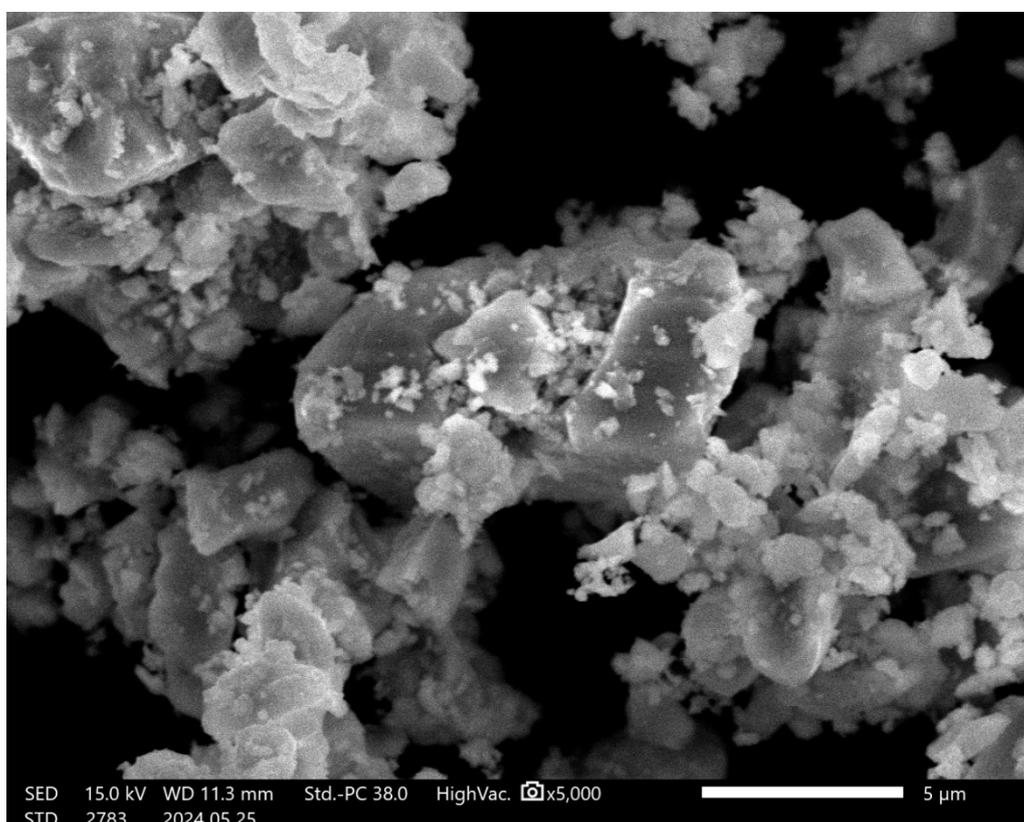
**Figure S2.** SEM image of  $\text{SrCa}_2\text{Ga}_2\text{O}_6:0.03\text{Mn}^{4+}$  powder after grinding.
