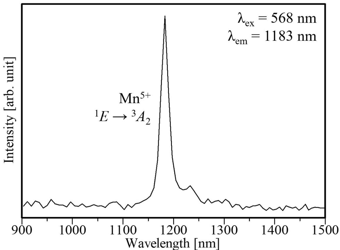
**Figure S4.** PL spectrum of tetrahedrally coordinated  $\text{Mn}^{5+}$  in  $\text{SrCa}_2\text{Ga}_2\text{O}_6:0.03\text{Mn}^{4+}$ .
