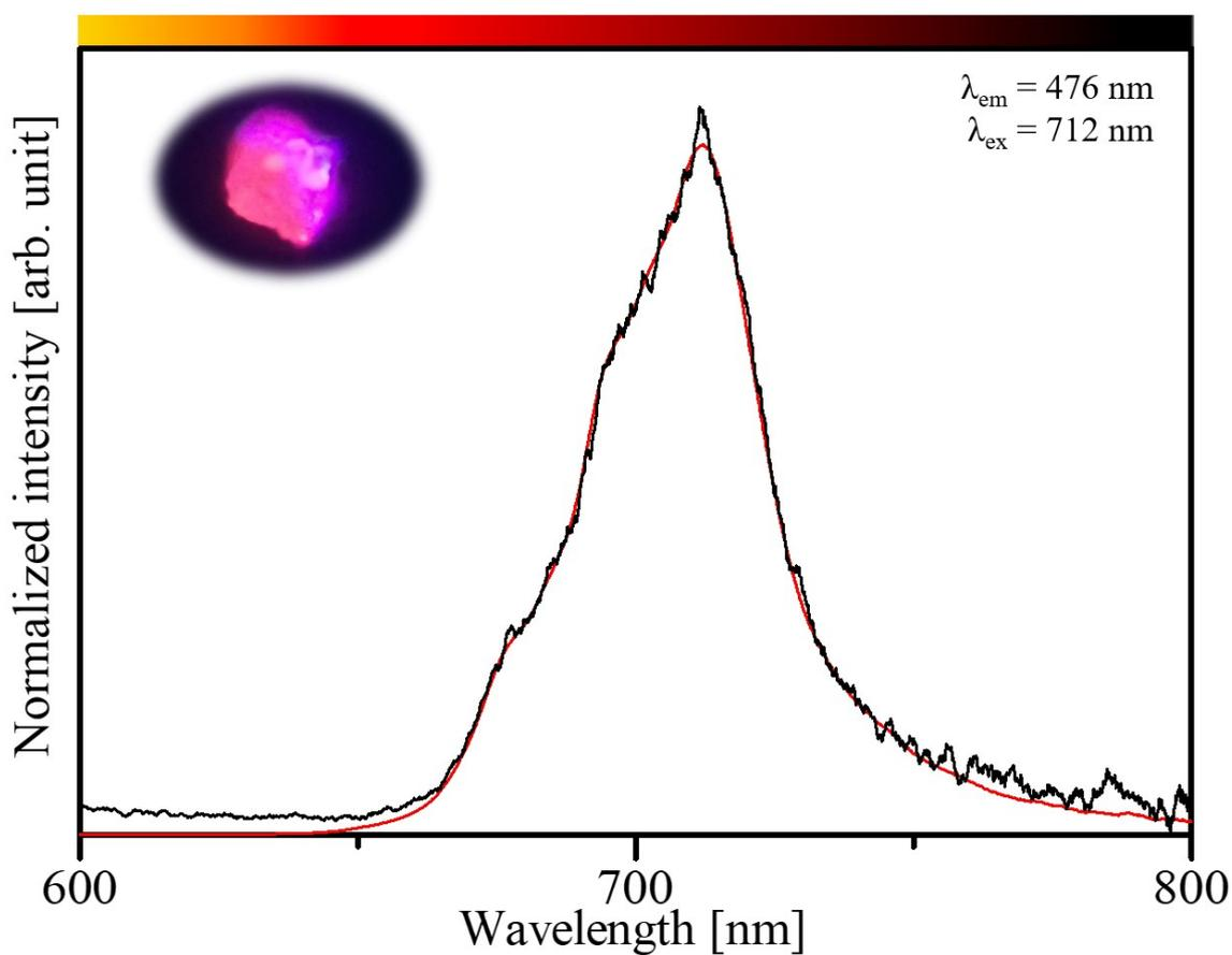
**Figure S1.** Normalized PL spectra of  $\text{SrCa}_2\text{Ga}_2\text{O}_6:\text{Mn}^{4+}$  single crystals (black line) and  $\text{SrCa}_2\text{Ga}_2\text{O}_6:0.03\text{Mn}^{4+}$  powder (red line). The insert photograph is the deep-red emitting  $\text{SrCa}_2\text{Ga}_2\text{O}_6:\text{Mn}^{4+}$  single crystal under 365 nm excitation
