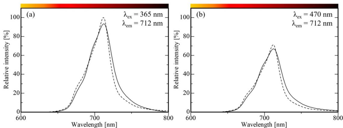
**Figure S3.** Normalized PL spectra of  $\text{SrCa}_2\text{Ga}_2\text{O}_6:0.03\text{Mn}^{4+}$  (solid lines) and  $\text{Ca}_{14}\text{Zn}_6\text{Ga}_{10}\text{O}_{35}:\text{Mn}^{4+}$  (dashed lines) phosphors excited by (a) 365 nm n-UV light and (b) 470 nm blue light.
