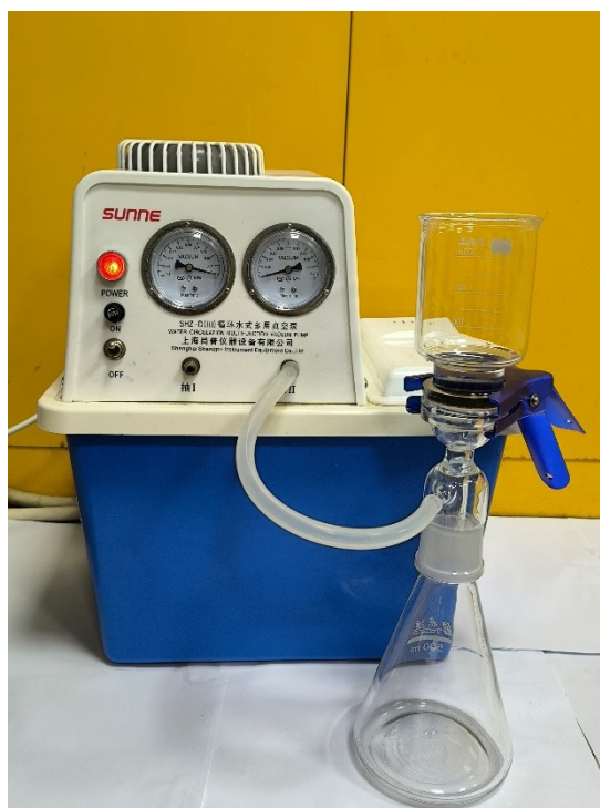
Fig. S1. Vacuum filtration system: The suction filter device is composed of SHZ-D(III) circulating water multi-purpose vacuum pump, Feida sand core suction filter device (300mL filter bowl, sand core filter head, 500mL receiving bottle, clip), and silicone connecting pipe.
