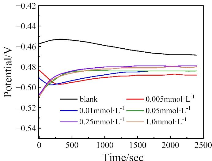
Figure S3. Open circuit potential versus time in  $1.0 \text{ mol}\cdot\text{L}^{-1}$  HCl solution containing different concentrations of PBT.
