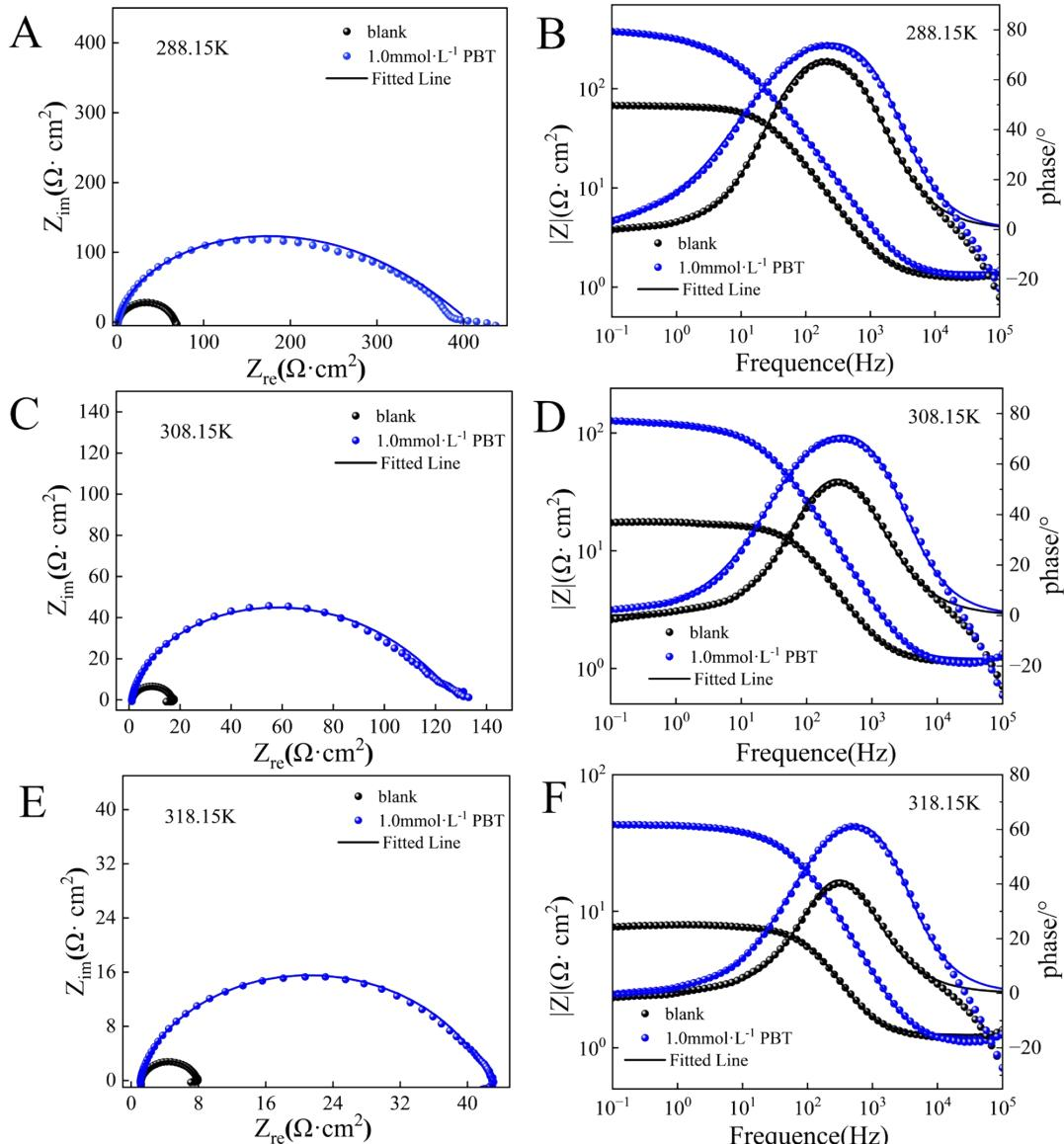
Figure S5 Nyquist plots (A, C and E) and Bode phase angle plots (B, D and F) for Q235 CS in 1.0 mol·L⁻¹ HCl with 1.0 mmol L⁻¹ of PBT at different temperature: 288.15K (A and B), 308.15K (C and D) and 318.15K (E and F).
