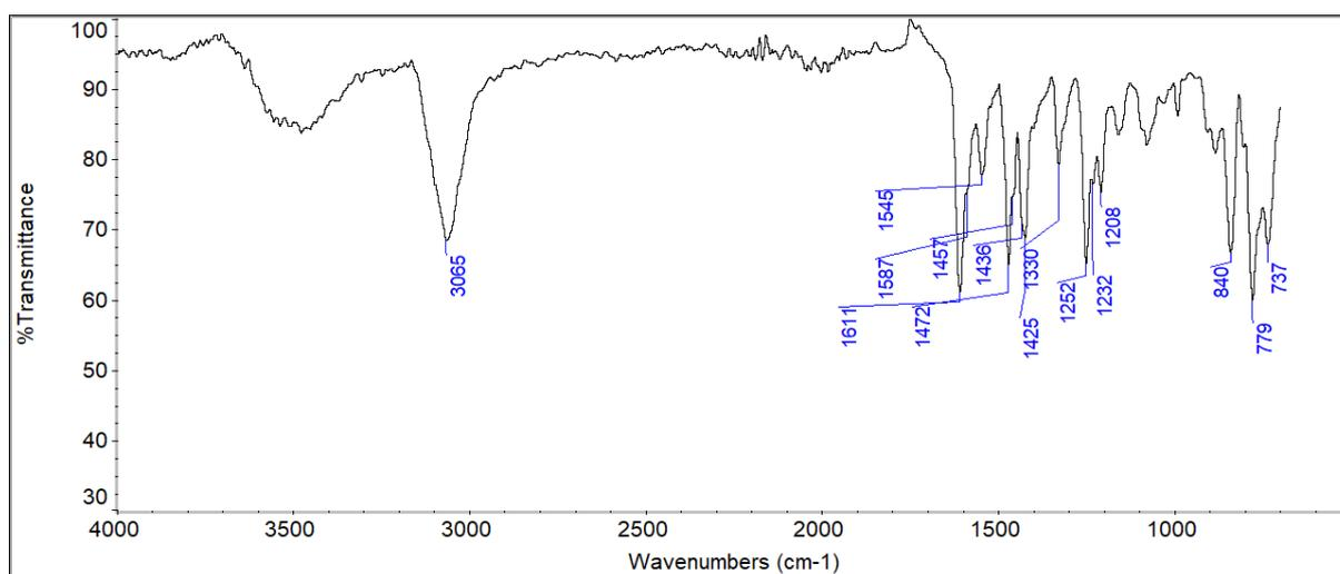
**Fig. S6** AT IR spectrum of **2**.
