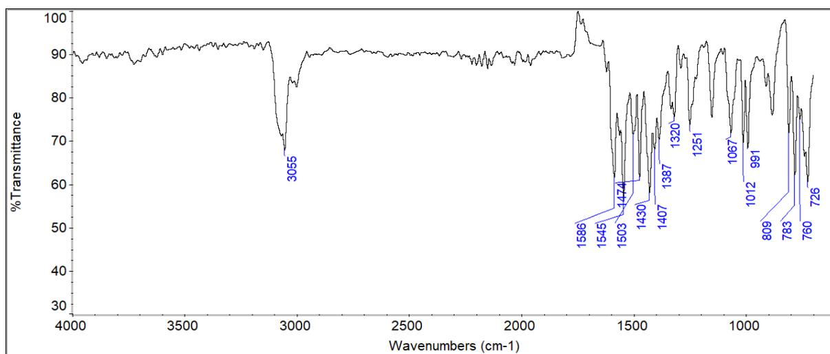
**Fig. S1** AT IR spectrum of the ligand **1**.
