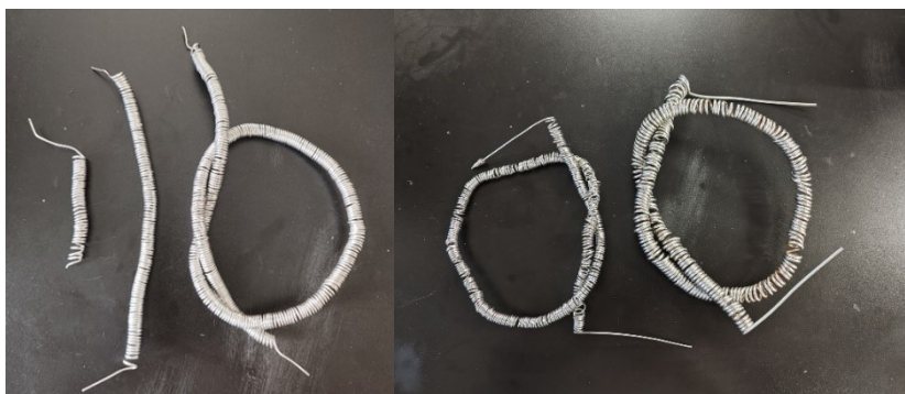
Figure S2 Physical drawing of 316L stainless steel reaction coil (left inner diameter 1 mm, length 1 m, 3 m, 10 m), 10 m inner diameter 0.65 mm, 10 m inner diameter 2 mm
