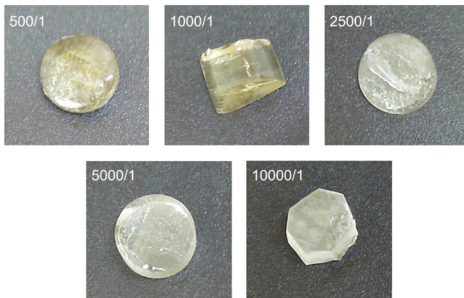
**Figure S5.** Various M/I p(HMNB) samples submerged in THF for four days.
