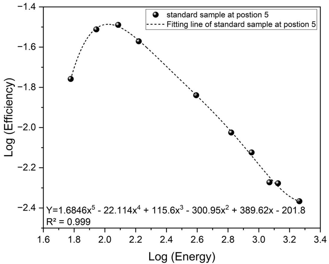
Figure S2. The relationship between energy and detection efficiency of standard sample at position 5.
