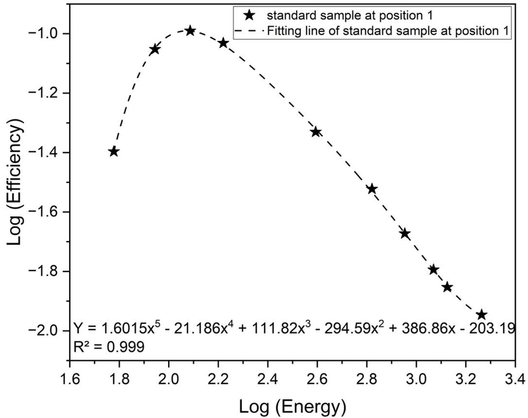
Figure S3. The relationship between energy and detection efficiency of standard sample at position 1.
