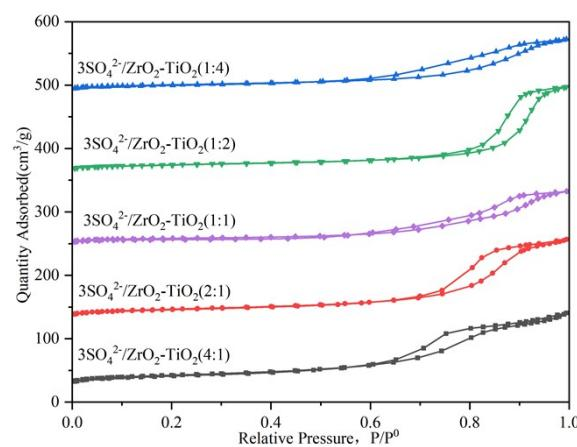
**Figure S1** N<sub>2</sub> adsorption and desorption isotherms of  $\text{SO}_4^{2-}/\text{ZrO}_2\text{-TiO}_2$  catalysts with different Zr/Ti molar ratios.
