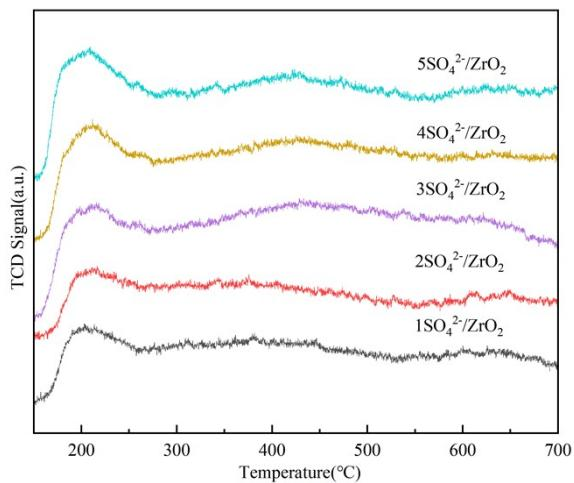
**Figure S2** NH<sub>3</sub>-TPD profiles of prepared catalysts
