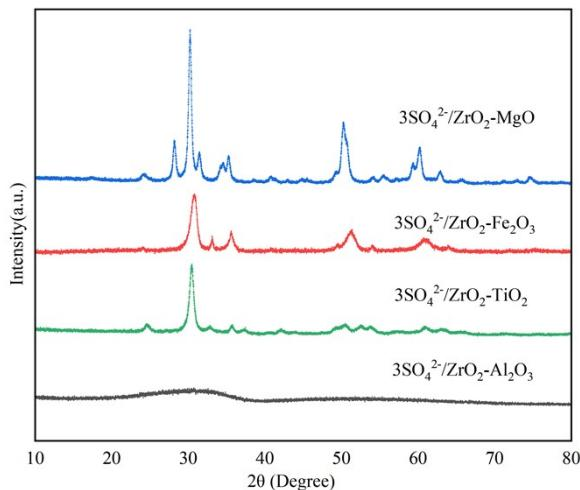
**Figure S3** XRD patterns of SO<sub>4</sub><sup>2-</sup>/ZrO<sub>2</sub> catalysts supported by different oxides
