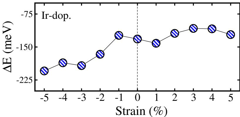
FIG. 7S: GGA+ $U$  computed energy difference ( $\Delta E = E_{\text{FIM}} - E_{\text{FM}}$ ) of the stable state ferrimagnetic (FIM) and ferromagnetic (FM) of the Ir-dop.  $\text{Sr}_2\text{CaOsO}_6$  double perovskite oxide as a function of  $\pm 5\%$  biaxial ([110]) strain.
