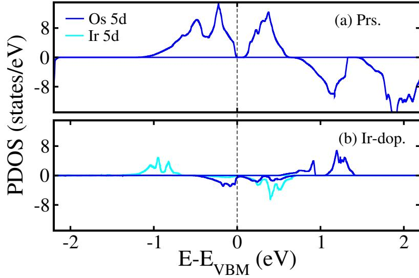
FIG. 3S: GGA+ $U$  computed non-degenerated 5d states resolved partial density of states (PDOS) projected on the Os/Ir ion in the (a) prs. and (b) Ir-dop.  $\text{Sr}_2\text{CaOsO}_6$  double perovskite oxides.
