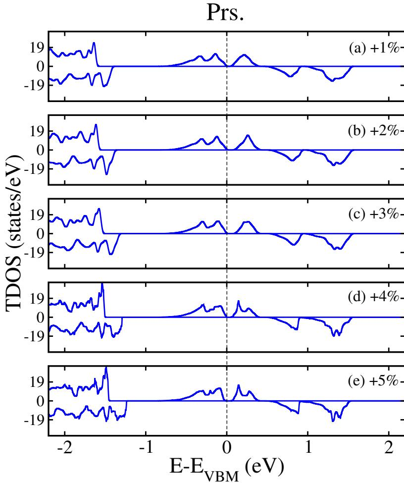
FIG. 8S: GGA+ $U$  Computed total density of states (TDOS) of the prs.  $\text{Sr}_2\text{CaOsO}_6$  double perovskite oxide as a function of (a) +1%, (b) +2%, (c) +3%, (d) +4%, and (e) +5% biaxial ([110]) tensile strains.
