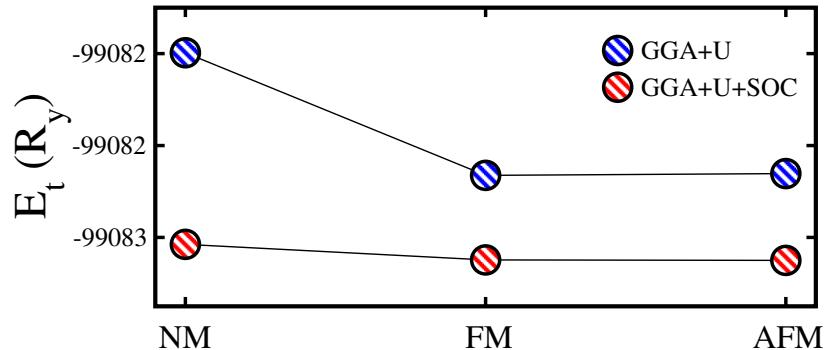
FIG. 2S: GGA+ $U$ /GGA+ $U$ +SOC computed total enrgy ( $E_t$ ) in the non-magnetic (NM), ferromagnetic (FM), and antiferromagnetic (AFM) spin ordering in the prs.  $\text{Sr}_2\text{CaOsO}_6$  double perovskite oxide.
