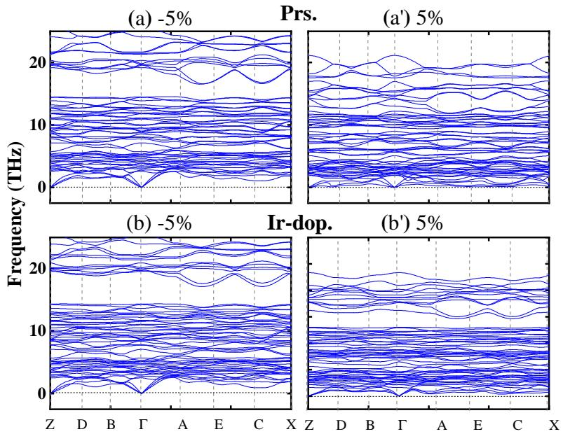
FIG. 6S: Computed phonon dispersion curves for the (a/b)  $-5\%$  and (a'/b')  $+5\%$  biaxial strains ([110]) in the prs./Ir-dop.  $\text{Sr}_2\text{CaOsO}_6$  double perovskite oxide.
