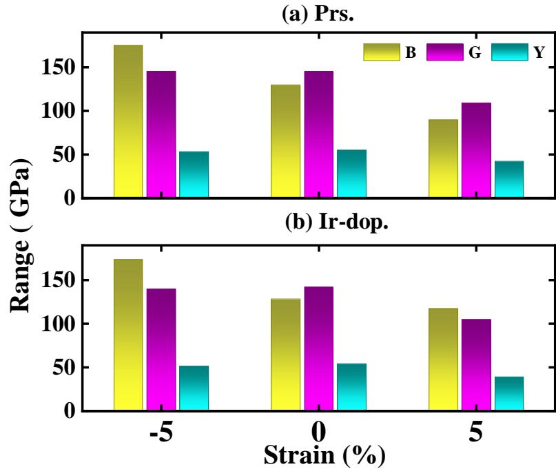
FIG. 1S: Computed Bulk modulus (B)/Shear modulus (G)/Youngs modulus (Y) for the (a) prs. and (b) Ir-dop.  $\text{Sr}_2\text{CaOsO}_6$  double perovskite oxides.
