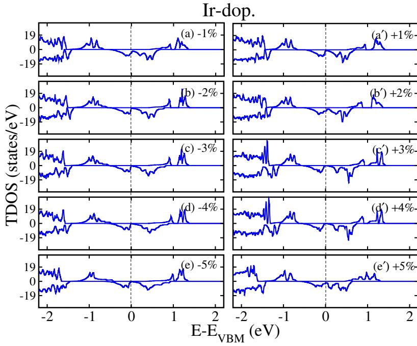
FIG. 9S: GGA+ $U$  computed total density of states (TDOS) of the Ir-dop.  $\text{Sr}_2\text{CaOsO}_6$  structure for the (a/a')  $-1/+1\%$ , (b/b')  $-2/+2\%$ , (c/c')  $-3/+3\%$ , (d/d')  $-4/+4\%$ , and (e/e')  $-5/+5\%$  biaxial ([110]) compressive/tensile strains.
