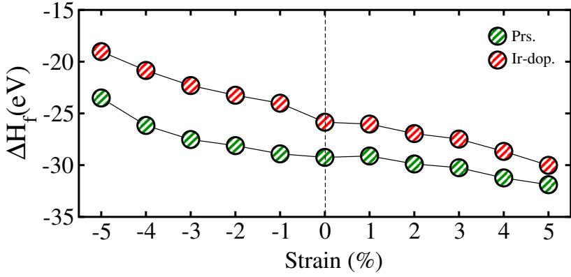
FIG. 5S: Computed formation enthalpy ( $\Delta H_f$ ) in the prs./Ir-dop.  $\text{Sr}_2\text{CaOsO}_6$  double perovskite oxide under  $\pm 5\%$  biaxial ([110]) strain.
