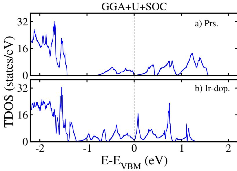
FIG. 4S: GGA+ $U$ +SOC computed non-degenerated total density of states (TDOS) in the (a) prs. and (b) Ir-dop.  $\text{Sr}_2\text{CaOsO}_6$  double perovskite oxides.
